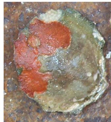
Figure A1.3: Old clock with hinge intact. No gloss on inner valve and heavy fouling.
