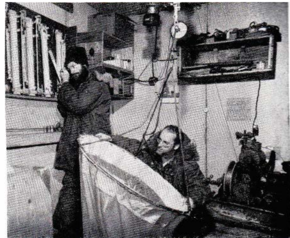
PL. 8. Interior of Station 61B, McMurdo Sound, showing a 1 m plankton net, Nansen bottles, and winch. Official U.S. Navy photograph
