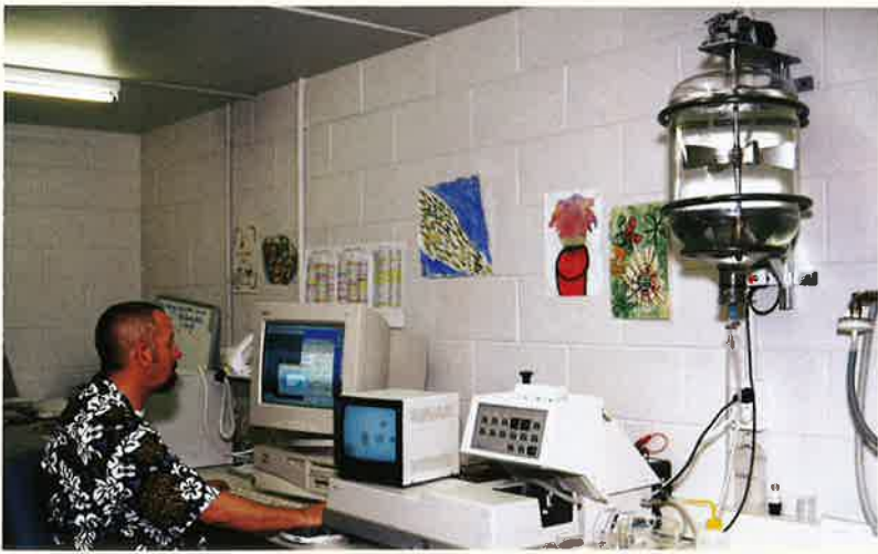
Galai instrument system for particle size and shape analysis.
