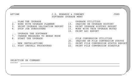
☐ Change messages to break mode. From the Software Upgrade Menu (A97IBM), select Change Messages to Break Mode.
