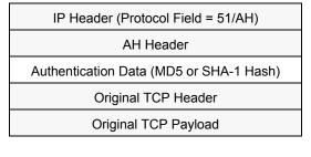
Authenticated data, note that TOS, Flags, Fragmentation, TTL, and Header Checksum fields of the IP Header are not covered by the authentication calculation.
