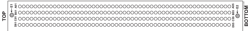
Figure B-31. Control Shelf HMUX A Pin-Outs
