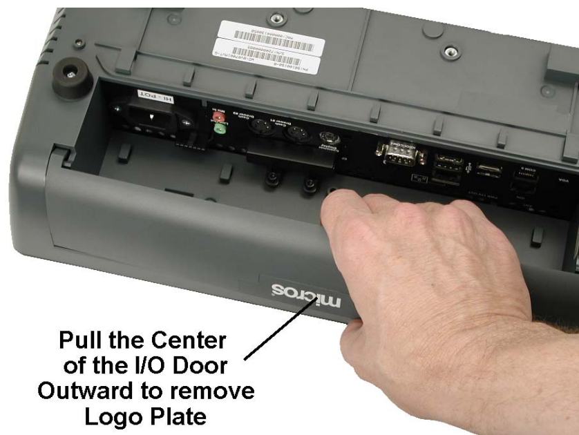
Figure 3-25: Removing the I/O Door
