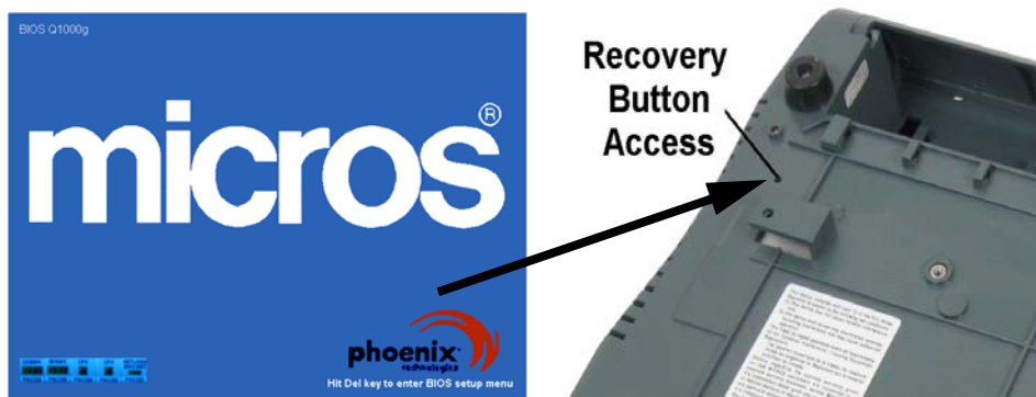
Figure 4-19: Press the Recovery Button when the Blue Splash Screen Appears
