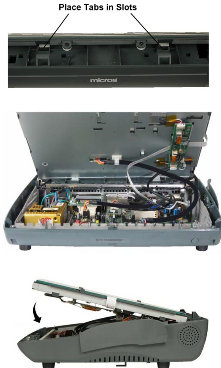
Figure 3-35: Installing the LCD/Touchscreen Assembly
