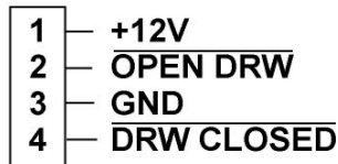
Figure B-6: Cash Drawer Connector Diagram
