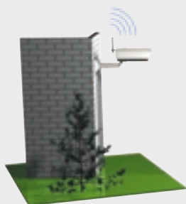
Camera in the wireless outdoor housing together with the universal outdoor wireless receiver.
