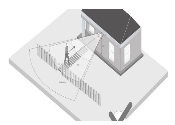
If the movement is detected very late, the object may not be completely visible on the video sequence.
