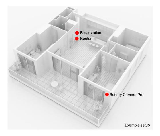
In an installation with two or more cameras, the base station should be placed as centrally as possible so that all cameras are within range of the base. The reception of the individual cameras is shown in the live view by means of the signal strength symbol.
