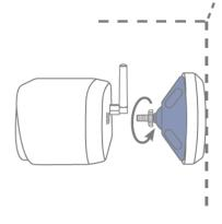
Insert the ball joint, fit the cover of the bracket and tighten. Then position the fixing ring and tighten slightly.
