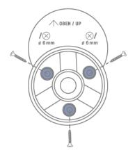
Mark three holes on a flat wall using the template, drill the holes (6 mm drill bit required) and attach the back plate of the bracket
