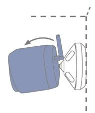
Turn the camera onto the thread of the ball head and align it with the desired detection area. Tighten the fixing ring in order to secure the camera in this position.
