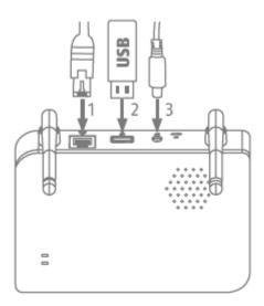
First plug in the network cable and the USB memory (with max. 128 GB storage capacity; not included in the scope of delivery). Then connect the power cable to the base station.
