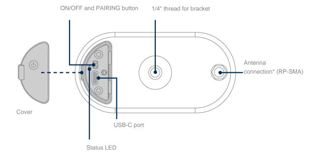
\*Wireless frequency: 2.4 GHz (802.11 b/g/n), max. transmission power 20 dBm
