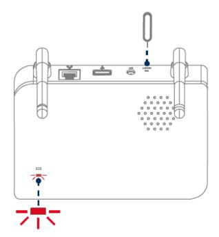
Reset to factory settings if necessary: Press and hold the reset button with the reset tool for 5 seconds until the power LED flashes red.
