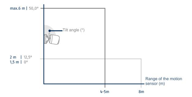
The higher the camera is installed, the greater the required downward tilt angle. This affects the range of the PIR sensor.
