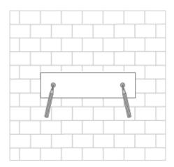
Install dowels and screws (see scope of delivery), then hook in the base station.
