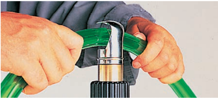
The reflector nozzle deflects the hot air for welding joints on plastic hoses
