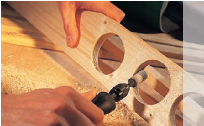
Routing with flexible drive in tight spaces
