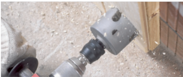
Multi Construction with Power Change adapter Page 163
