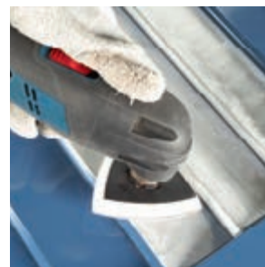
Sanding down, conditioning and polishing varnish with the sanding sheet sets and polishing pads.
