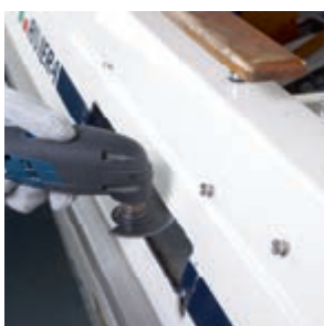
Cutting epoxy and fibreglass is also possible with the new diamond blade; longest lifetime, e.g. for a ventilation grille in a boat's hull.
