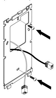
Mount the bracket to the wall so the Telco Box is ready available behind the mounting plate.
