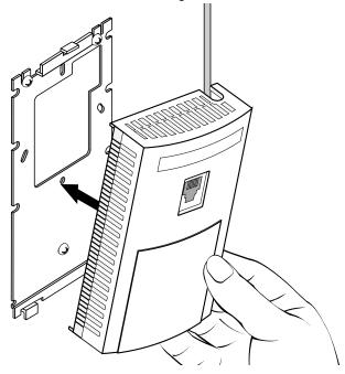
Once installed, connections are hidden from forward view, with only the physical infrastructure cables (Ethernet and power) extending from the Access Point.
