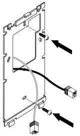
2. Connect one end of an RJ-45 cable into the wall mount connector on the Access Point as illustrated below.
