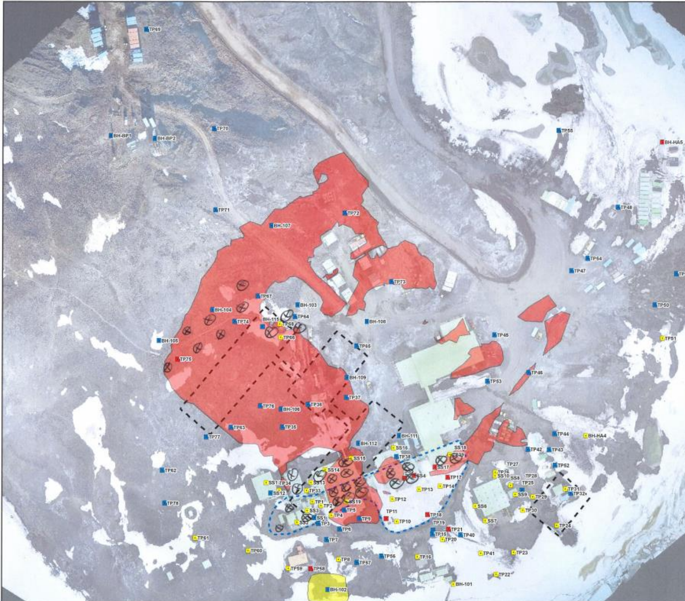
Figure 30. The excavation sites will be around the current base, down towards the foreshore and along the Hillary Trail. Each excavation site will disturb an area of around 4m in diameter. The Scott Base excavator will be used for this work.
