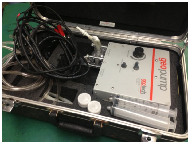
Figure 4. Electric pump and syringes used to contrast filtering methods.
