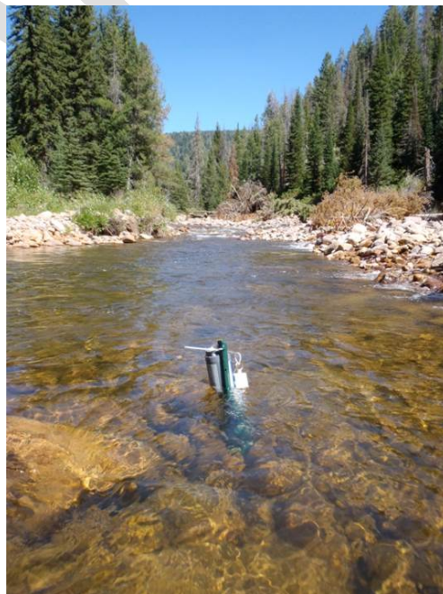
Photo 3.1. Example of a water quality probe.
