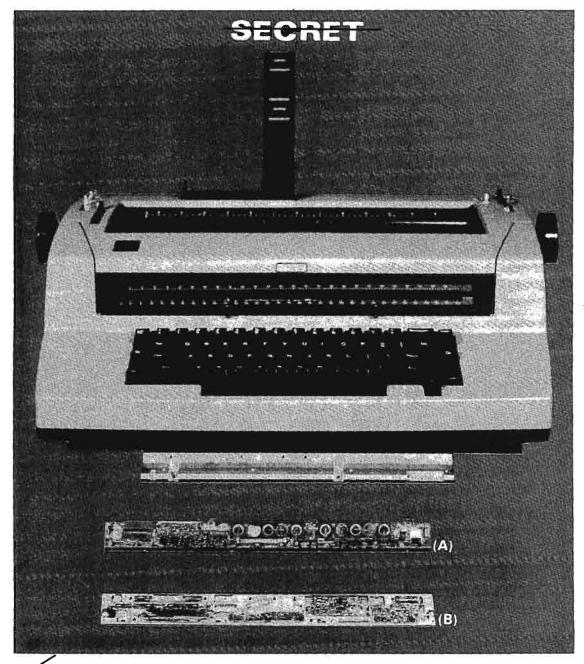
(8) One of the Gunman typewriters. Under it is the bar, both assembled and disassembled to show the embedded electronics.
