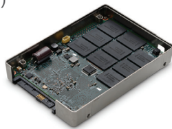
1920GB, 1600GB, 1000GB, 800GB, 500GB, 400GB and 250GB MLC | 2.5-inch SFF | SAS 12Gb/s
