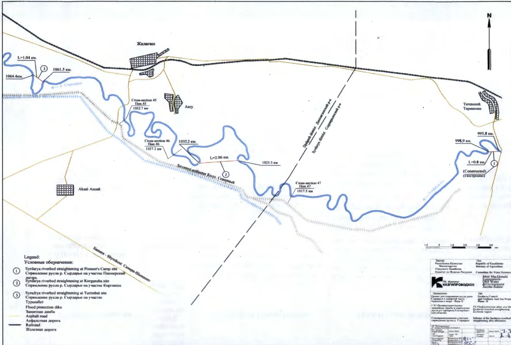
Scheme of the Syrdarya riverbed straightening' at Korgansha and Turumbet sites
