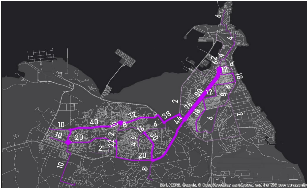
Above: number of vehicles per hour, average at peak – 6 AM to 8 AM
