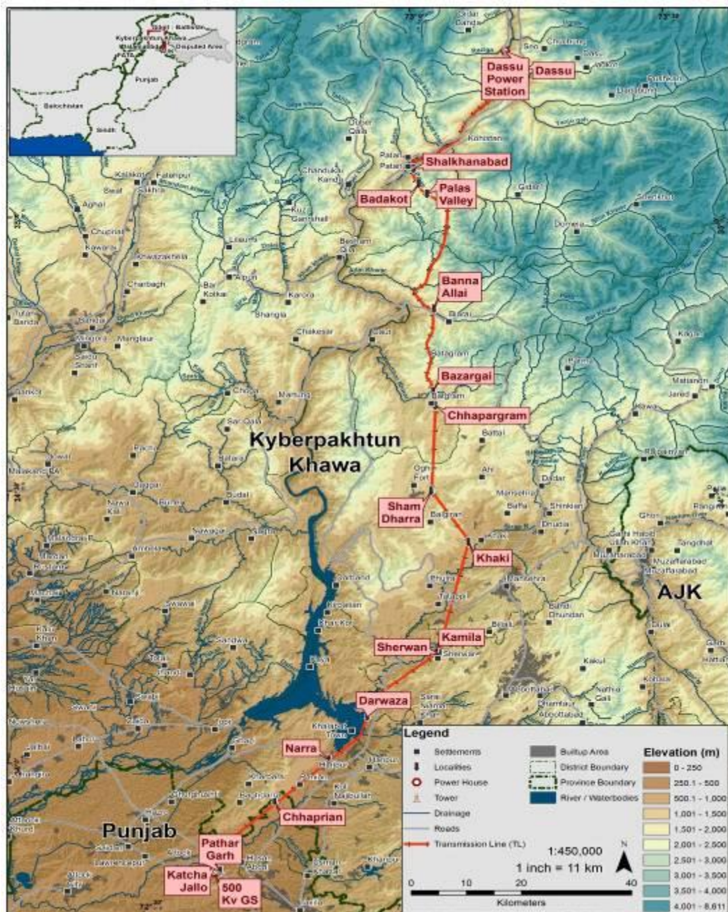
Figure 3.6: Proposed Alignment of Transmission Lines
