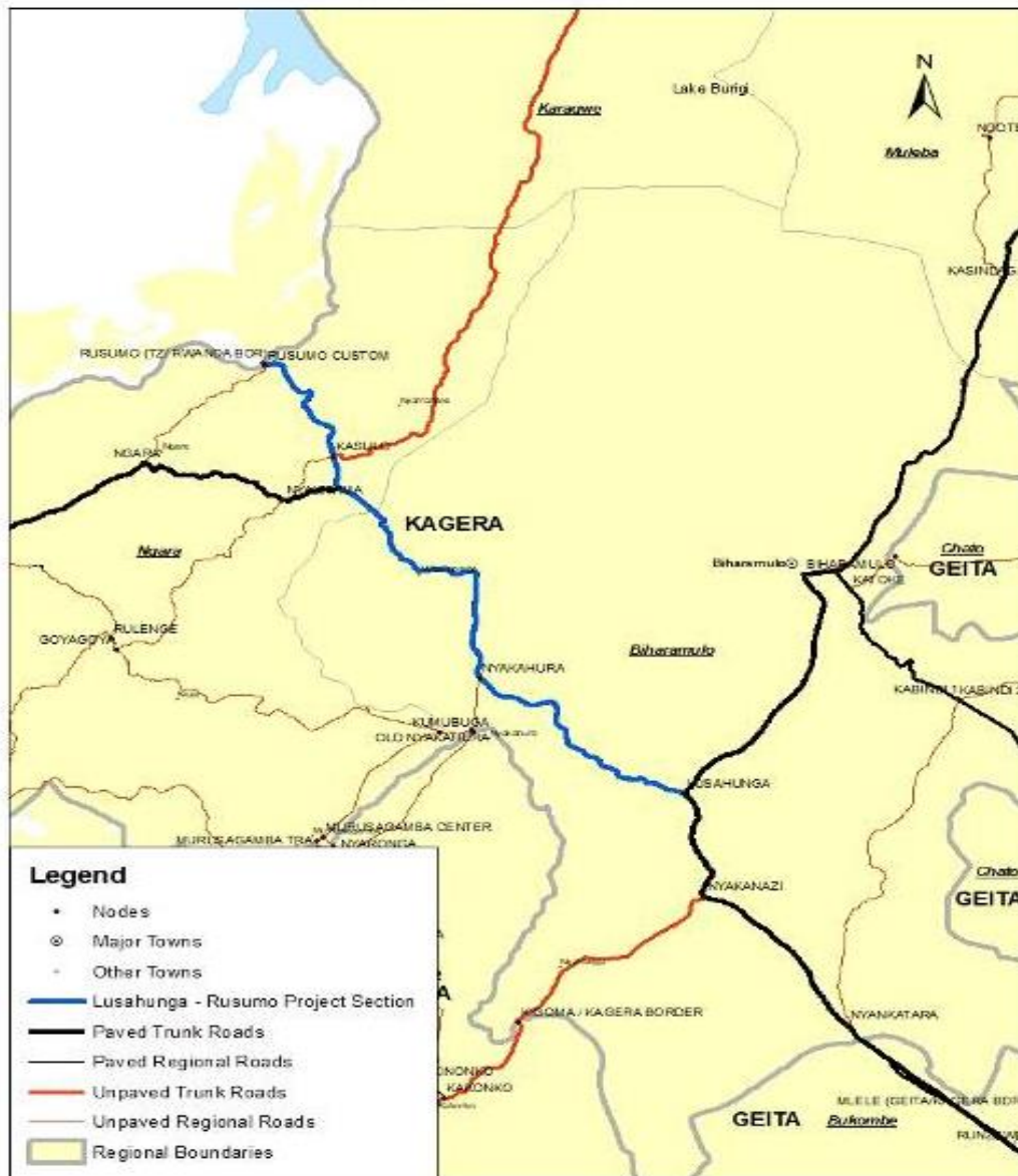
Figure 2-3 Road Network Map showing project road
