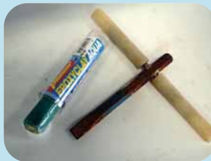
A stick of two-part epoxy putty and hand-auger made by welding a steel handle to a cold chisel and covering the handle with plastic tube (P. Cabaitan).
