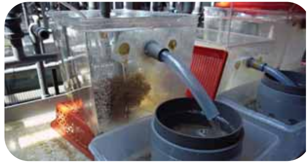
Ex situ larval collection using an overflow pipe and mesh collector (J. Guest).
