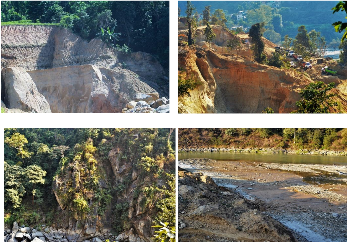
Figure 4-4: Alluvial and residual soil types in the open deposit area along existing Highway
