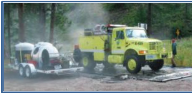
Figure 6. A portable washer to clean vehicles in challenging terrain. The system fits on a trailer and can be towed by a pickup truck. It reuses wash water and is inexpensive 2
