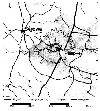
Figure 6-3: Highest hourly SO<sub>2</sub> predicted ground level concentrations due to future operational conditions (300 m stack height)
