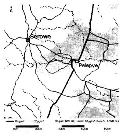
Figure 6-11: Annual average SO<sub>2</sub> predicted ground level concentrations due to future operational conditions 300 m stack height
