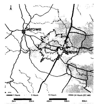
Figure 6-4: Frequency of exceedance of the hourly  $SO_2$  predicted ground level concentrations (based on the EC allowable exceedance of the 350 µg/m<sup>3</sup> of 24 hours per year) - future at 150 m stack height
