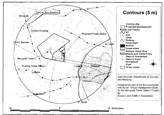
Figure 6: Contours (5m) and expected flow of cold air (Source Surveys and Mapping)
