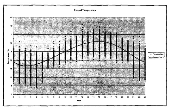
Figure 4-5: Diurnal temperature variation based on simulated data for Morupule for the year 2005.
