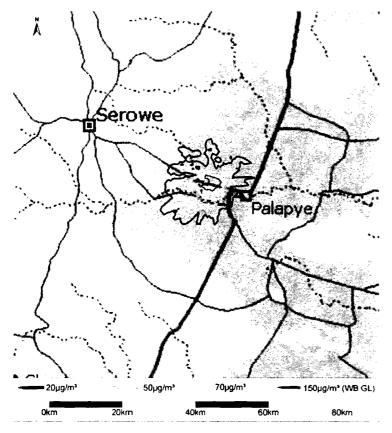
Figure 6-15: Highest daily average PM10 predicted ground level concentrations due to future operational conditions (150 m stack)
