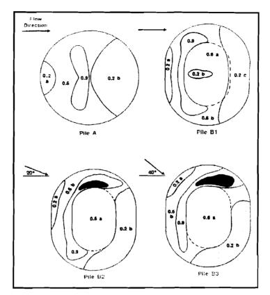
Figure A- 2: Contours of normalised surface wind speeds (i.e. surface wind speed / approach wind speed) (after EPA, 1998c).
