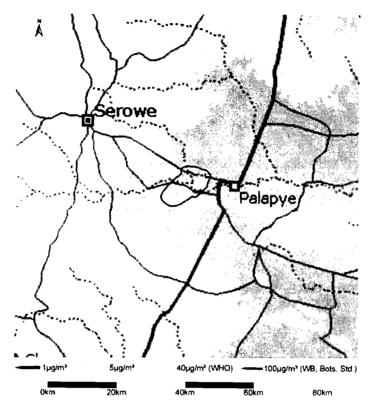
Figure 6-14: Annual average NO<sub>2</sub> predicted ground level concentrations due to future operational conditions (150 m stack)
