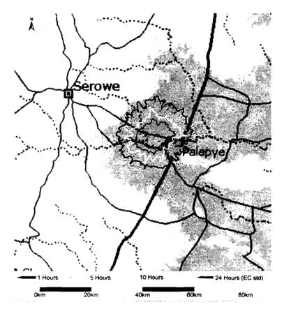
Figure 5-3: Frequency of exceedance of the hourly  $SO_2$  predicted ground level concentrations (based on the EC allowable exceedance of the 350 µg/m<sup>3</sup> of 24 hours per year) - baseline
