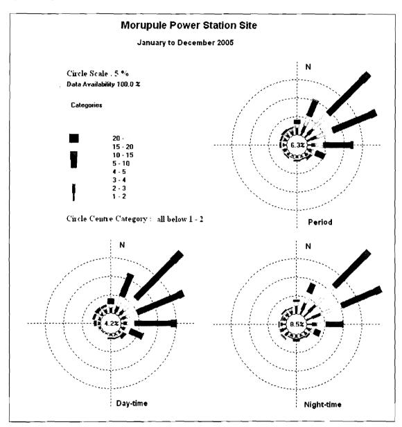
Figure 4-3: Day-time, night-time and period average wind roses for the simulated on-site wind field for the period 2005
