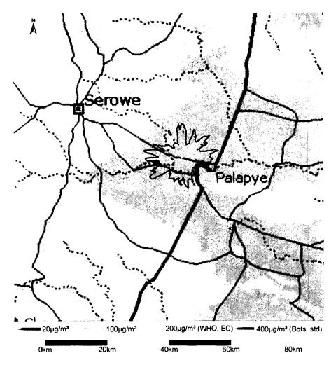
Figure 5-7: Highest hourly NO<sub>2</sub> predicted ground level concentrations due to baseline conditions
