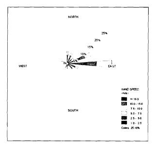
Figure 4-2: Wind rose reflecting the 2 months on-site meteorological data (May to June 2007)
