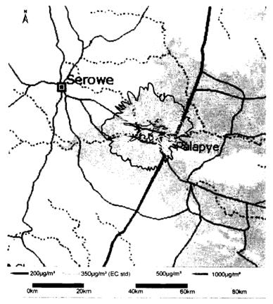
Figure 5-2: Highest hourly SO<sub>2</sub> predicted ground level concentrations due to baseline conditions
