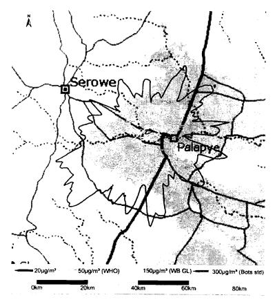
Figure 6-6: Highest daily average SO<sub>2</sub> predicted ground level concentrations due to future operational conditions at 200 m stack height
