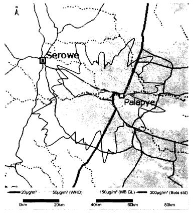
Figure 6-5: Highest daily average SO<sub>2</sub> predicted ground level concentrations due to future operational conditions at 150 m stack height
