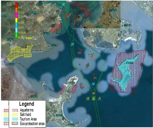
Figure 8.4.19 Impact Scope of Oil Spill Accident Occurred at Point A in Ebb Slack Period in Case of a SSW Wind (after 3-9 hours)
