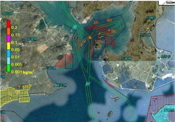
Figure 8.4.52 Impact Scope of Oil Spill Accident Occurred at Point C in Ebb Slack Period in Case of Calm Wind (after 3-12 hours)
