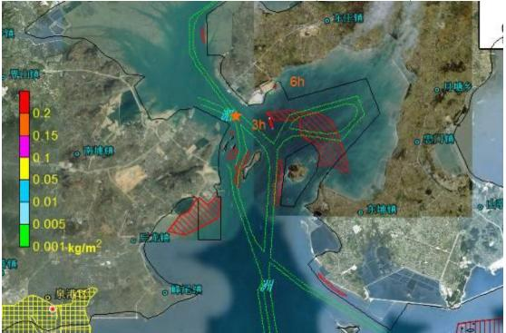
Figure 8.4.102 Impact Scope of Oil Spill Accident Occurred at Point D in Ebb Tide Period in Case of a SSW Wind (after 3-6 hours)
