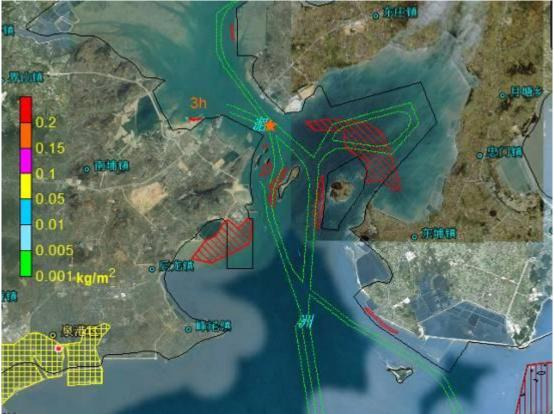
Figure 8.4.98 Impact Scope of Oil Spill Accident Occurred at Point D in Flood Tide Period in Case of a NE Wind (after 3 hours)
