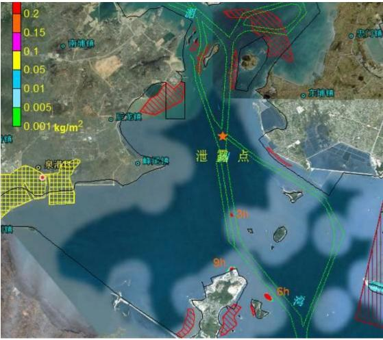
Figure 8.4.40 Impact Scope of Oil Spill Accident Occurred at Point B in Flood Slack Period in Case of a NE Wind (after 3-9 hours)
