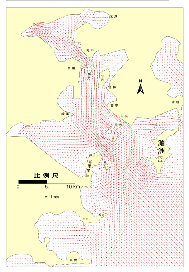
Figure 6.2-10 Up rapids flow field at flood tide following channel dredging
