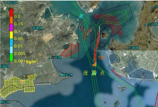
Figure 8.4.25 Impact Scope of Oil Spill Accident Occurred at Point B in Ebb Slack Period in Case of Calm Wind (after 12 hours)
