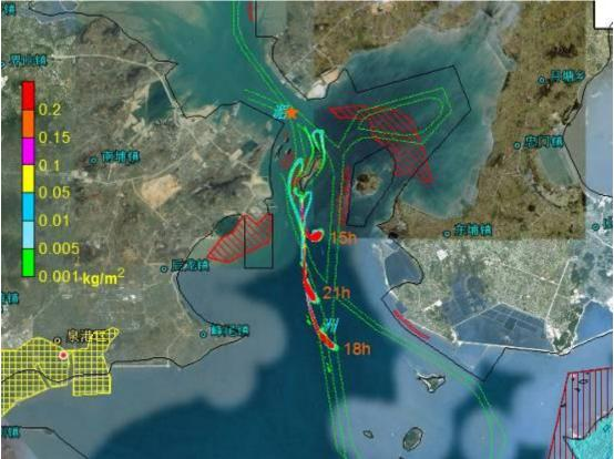
Figure 8.4.76 Impact Scope of Oil Spill Accident Occurred at Point D in Flood Slack Period in Case of Calm Wind (after 15-21 hours)
