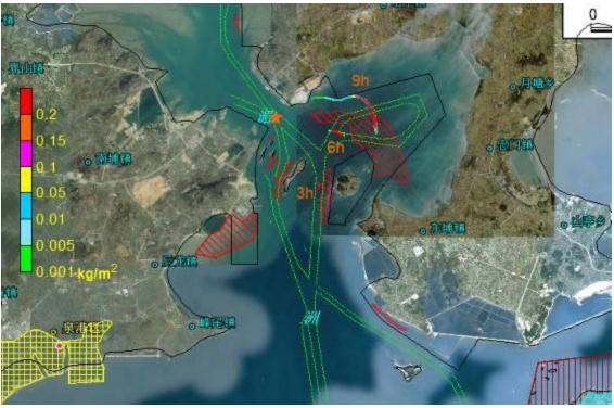
Figure 8.4.91 Impact Scope of Oil Spill Accident Occurred at Point D in Ebb Tide Period in Case of Calm Wind (after 3-9 hours)
