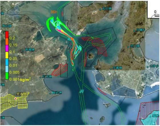
Figure 8.4.79 Impact Scope of Oil Spill Accident Occurred at Point D in Flood Slack Period in Case of Calm Wind (after 36 hours)
