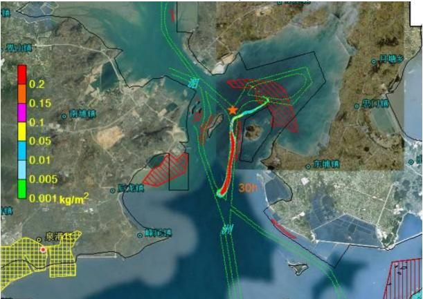
Figure 8.4.66 Impact Scope of Oil Spill Accident Occurred at Point C in Ebb
