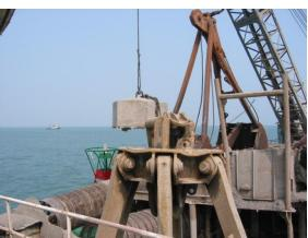
Grab bucket sludge-carrying vessel and the hopper barge
