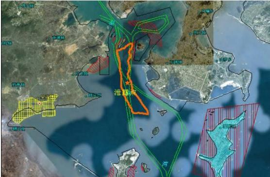
Figure 8.4.109 Maximum Impact Scope of Oil Spill Accident Occurred at Point B in Flood Tide Period After 36 Hours in Case of Calm Wind
