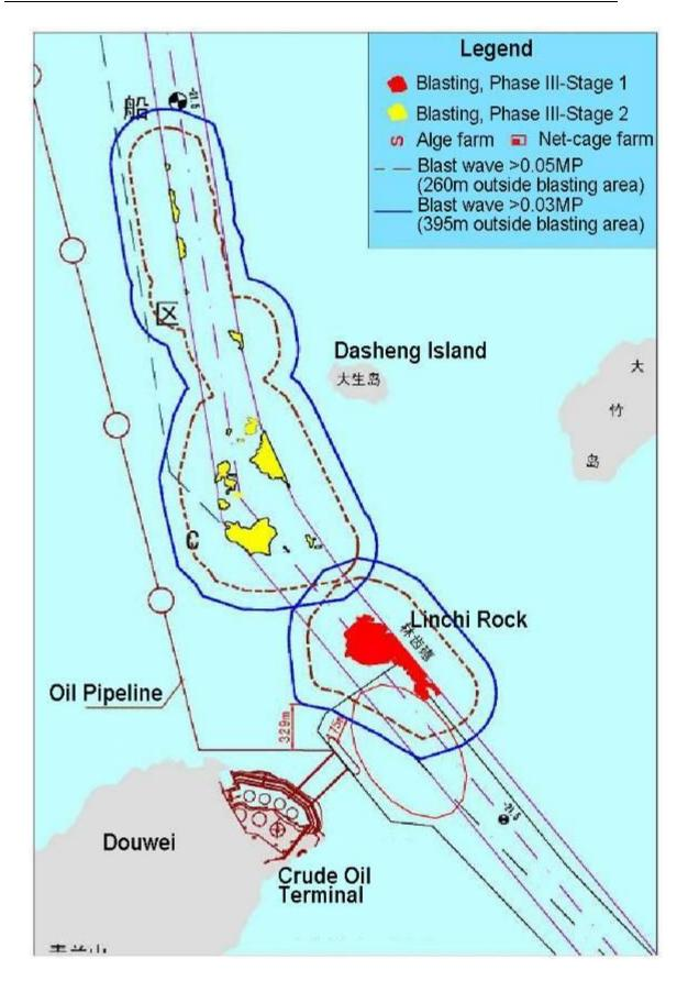
Figure 6.1.7 Impact range of blast waves from the main channel rock blasting areas near Dasheng Island
