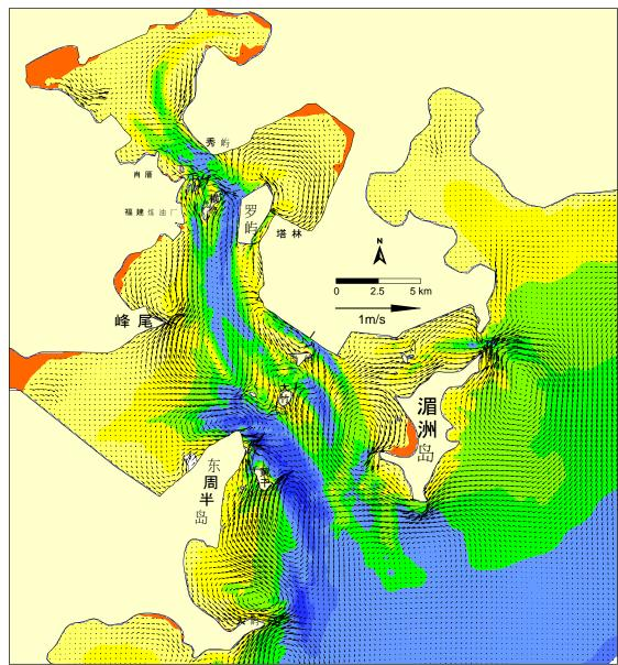
Figure 6.2-6 Flow field of tide-induced residual currents before construction
