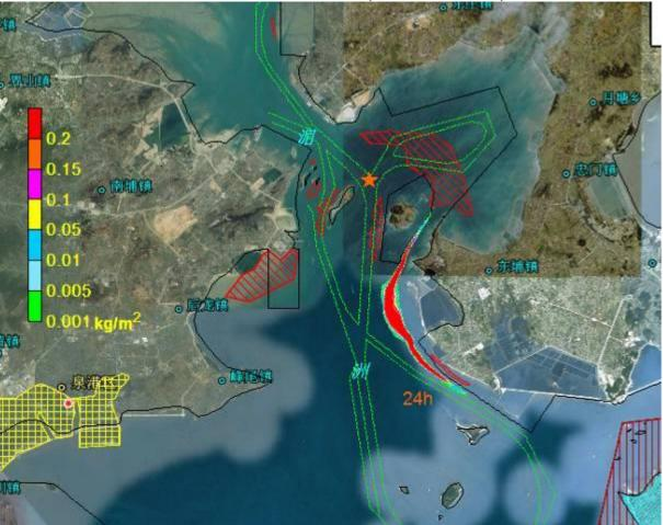
Figure 8.4.54 Impact Scope of Oil Spill Accident Occurred at Point C in Ebb
