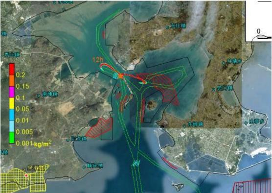
Figure 8.4.84 Impact Scope of Oil Spill Accident Occurred at Point D in Flood Tide Period in Case of Calm Wind (after 12 hours)
