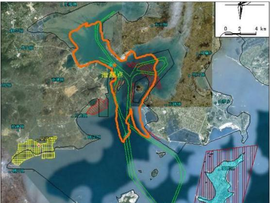
Figure 8.4.117 Maximum Impact Scope of Oil Spill Accident Occurred at Point D in Flood Tide Period After 36 Hours in Case of Calm Wind
