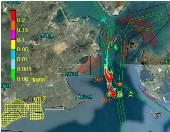
Figure 8.4.39 Impact Scope of Oil Spill Accident Occurred at Point B in Ebb Tide Period in Case of Calm Wind (after 30-36 hours)
