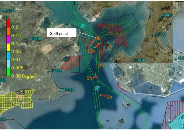
Figure 8.4.49 Impact Scope of Oil Spill Accident Occurred at Point C in Flood Slack Period in Case of Calm Wind (after 3-12 hours)
