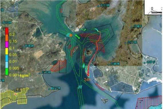
Figure 8.4.94 Impact Scope of Oil Spill Accident Occurred at Point D in Ebb Tide Period in Case of Calm Wind (after 24 hours)
