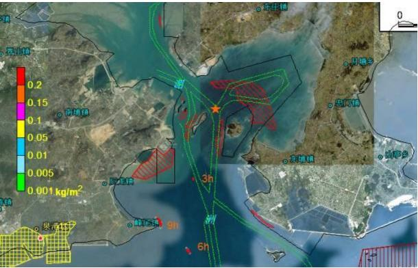
Figure 8.4.68 Impact Scope of Oil Spill Accident Occurred at Point C in Flood Slack Period in Case of a NE Wind (after 3-9 hours)
