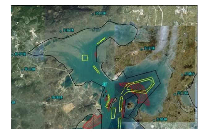
Figure 6.1-1 Layout 1 of calculation points in dredging simulation
