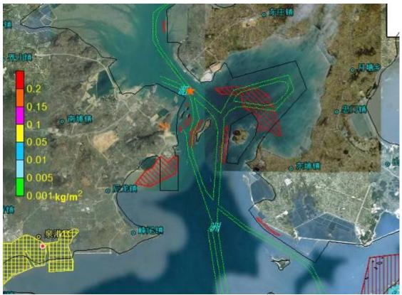
Figure 8.4.97 Impact Scope of Oil Spill Accident Occurred at Point D in Flood Slack Period in Case of a NE Wind (after 3 hours)
