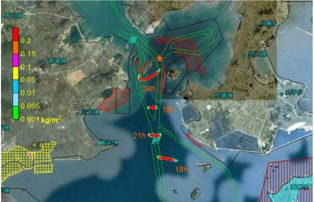
Figure 8.4.50 Impact Scope of Oil Spill Accident Occurred at Point C in Flood Slack Period in Case of Calm Wind (after 15-24 hours)
