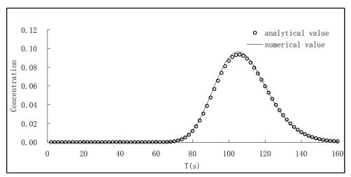
Figure 8.5.3 Concentration Development Curve at Coordinate (100,80) under the Second Group of Diffusion Parameters
