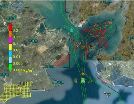
Figure 8.4.45 Impact Scope of Oil Spill Accident Occurred at Point B in Ebb Slack Period in Case of a SSW Wind (after 3-9 hours)
