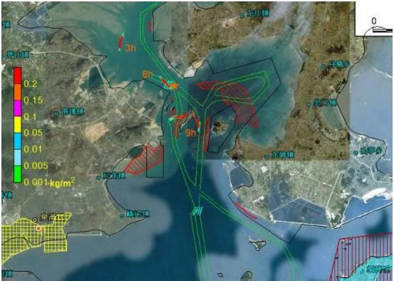
Figure 8.4.83 Impact Scope of Oil Spill Accident Occurred at Point D in Flood Tide Period in Case of Calm Wind (after 3-9 hours)
