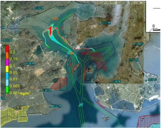
Figure 8.4.85 Impact Scope of Oil Spill Accident Occurred at Point D in Flood Tide Period in Case of Calm Wind (after 15 hours)
