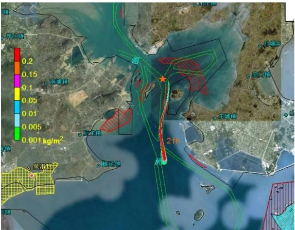
Figure 8.4.59 Impact Scope of Oil Spill Accident Occurred at Point C in Flood Tide Period in Case of Calm Wind (after 21 hours)
