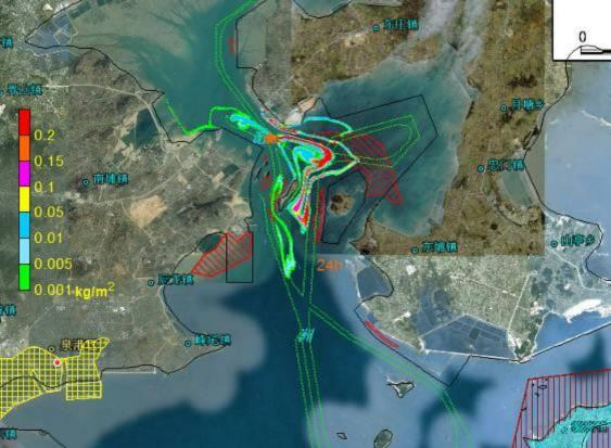
Figure 8.4.88 Impact Scope of Oil Spill Accident Occurred at Point D in Flood Tide Period in Case of Calm Wind (after 24 hours)
