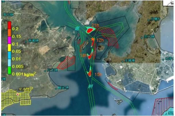
Figure 8.4.64 Impact Scope of Oil Spill Accident Occurred at Point C in Ebb Tide Period in Case of Calm Wind (after 12-21 hours)
