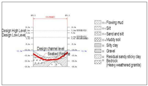
Figure 6.1-11 Vertical position of pipeline at the Putou channel area
