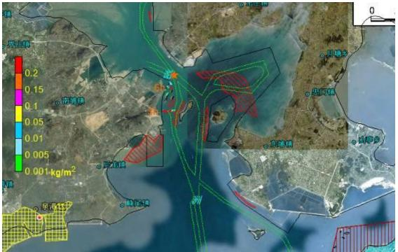
Figure 8.4.99 Impact Scope of Oil Spill Accident Occurred at Point D in Ebb Tide Period in Case of a NE Wind (after 3-6 hours)
