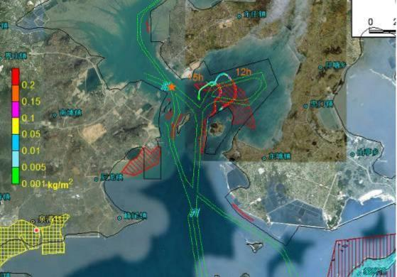
Figure 8.4.92 Impact Scope of Oil Spill Accident Occurred at Point D in Ebb Tide Period in Case of Calm Wind (after 12-15 hours)
