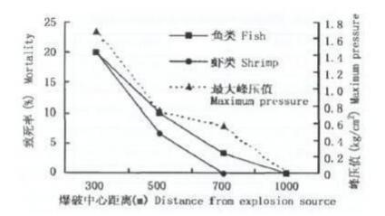
Figure 6.1-5 Relation between the explosion-induced mortality of marine life and the distance from explosion source
