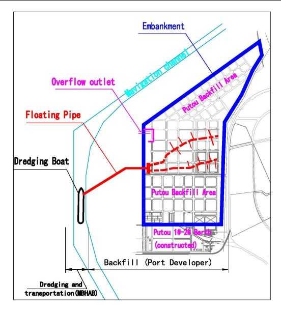
Figure 3.2-3 Backfilling (reclamation) operation
