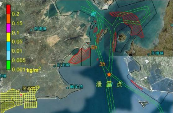
Figure 8.4.41 Impact Scope of Oil Spill Accident Occurred at Point B in Ebb
