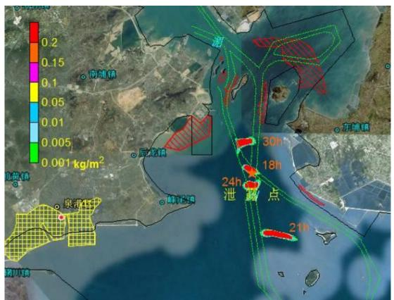
Figure 8.4.34 Impact Scope of Oil Spill Accident Occurred at Point B in Flood Tide Period in Case of Calm Wind (after 18-30 hours)
