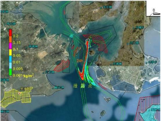
Figure 8.4.29 Impact Scope of Oil Spill Accident Occurred at Point B in Ebb
