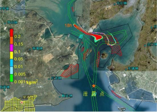
Figure 8.4.27 Impact Scope of Oil Spill Accident Occurred at Point B in Ebb Slack Period in Case of Calm Wind (after 18 hours)
