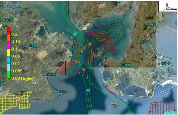
Figure 8.4.70 Impact Scope of Oil Spill Accident Occurred at Point C in Ebb Tide Period in Case of a NE Wind (after 3-6 hours)
