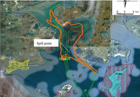
Figure 8.4.108 Maximum Impact Scope of Oil Spill Accident Occurred at Point B in Ebb Slack Period After 36 Hours in Case of Calm Wind
