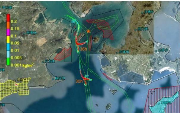
Figure 8.4.51 Impact Scope of Oil Spill Accident Occurred at Point C in Flood Slack Period in Case of Calm Wind (after 30-36 hours)
