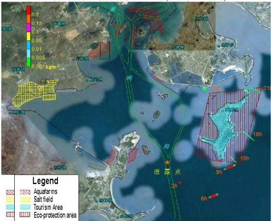
Figure 8.4.18 Impact Scope of Oil Spill Accident Occurred at Point A in Flood Slack Period in Case of a SSW Wind (after 3-24 hours)
