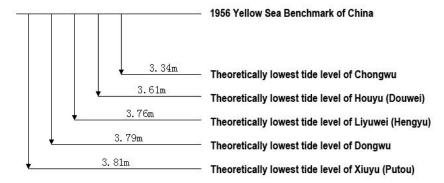
Figure 5.1-1 Conversion Relationship between tidal level and basal plane
