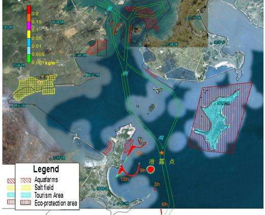
Figure 8.4.13 Impact Scope of Oil Spill Accident Occurred at Point A in Flood
