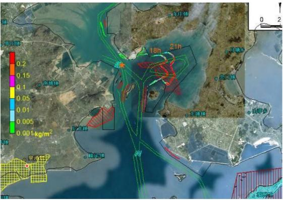
Figure 8.4.93 Impact Scope of Oil Spill Accident Occurred at Point D in Ebb Tide Period in Case of Calm Wind (after 18-21 hours)
