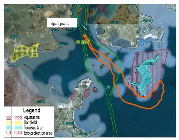
Figure 8.4.107 Maximum Impact Scope of Oil Spill Accident Occurred at Point B in Flood Slack Period After 36 Hours in Case of Calm Wind
