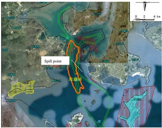
Figure 8.4.110 Maximum Impact Scope of Oil Spill Accident Occurred at Point B in Ebb Tide Period After 36 Hours in Case of Calm Wind
