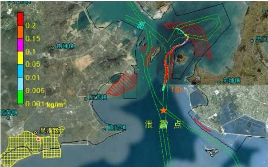
Figure 8.4.26 Impact Scope of Oil Spill Accident Occurred at Point B in Ebb Slack Period in Case of Calm Wind (after 15 hours)
