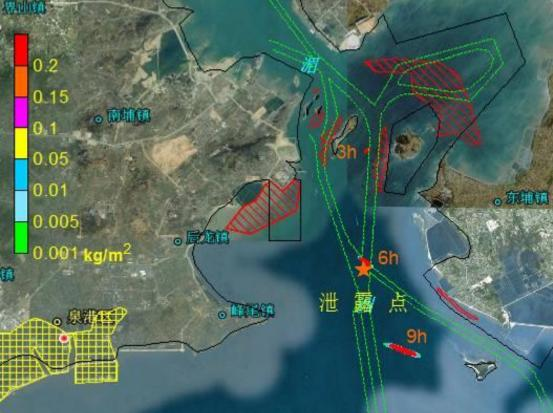
Figure 8.4.32 Impact Scope of Oil Spill Accident Occurred at Point B in Flood Tide Period in Case of Calm Wind (after 3-9 hours)
