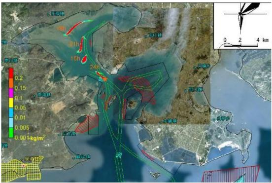
Figure 8.4.81 Impact Scope of Oil Spill Accident Occurred at Point D in Ebb Slack Period in Case of Calm Wind (after 15-24 hours)
