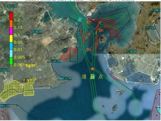
Figure 8.4.24 Impact Scope of Oil Spill Accident Occurred at Point B in Ebb Slack Period in Case of Calm Wind (after 3-9 hours)
