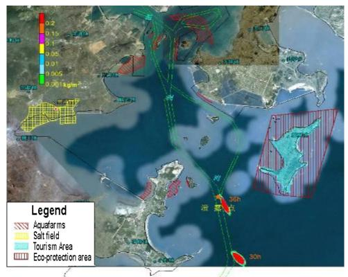
Figure 8.4.4 Impact Scope of Oil Spill Accident Occurred at Point A in Flood Slack Period in Case of Calm Wind (after 30-36 hours)
