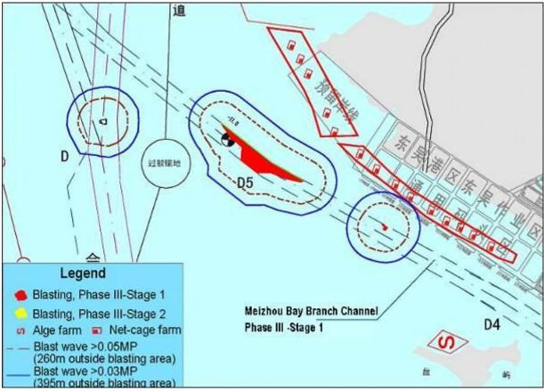
Figure 6.1.8 Impact range of blast waves from rock blasting areas at the main channel and branch channel
