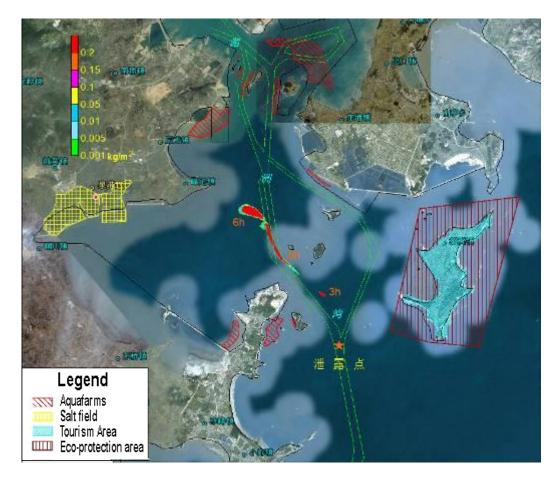
Figure 8.4.5 Impact Scope of Oil Spill Accident Occurred at Point A in Ebb Slack Period in Case of Calm Wind (after 3-9 hours)
