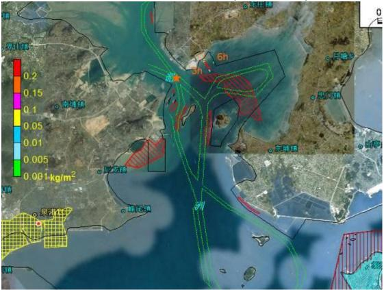
Figure 8.4.100 Impact Scope of Oil Spill Accident Occurred at Point D in Flood Slack Period in Case of a SSW Wind (after 3-6 hours)
