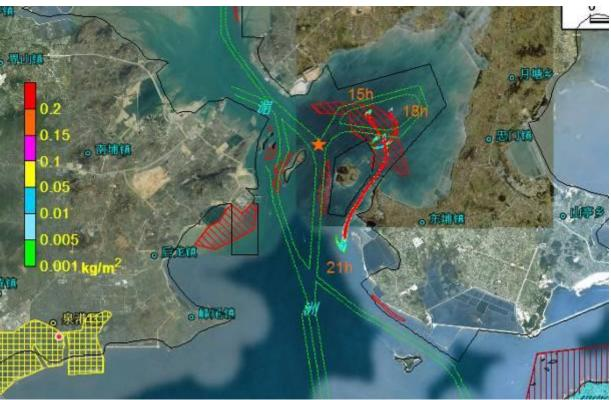
Figure 8.4.53 Impact Scope of Oil Spill Accident Occurred at Point C in Ebb Slack Period in Case of Calm Wind (after 15-21 hours)
