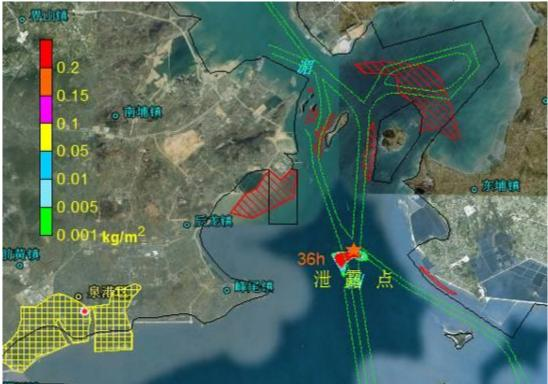
Figure 8.4.35 Impact Scope of Oil Spill Accident Occurred at Point B in Flood
