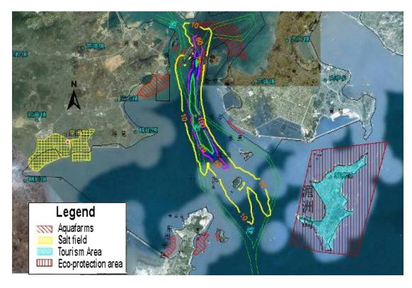
Figure 8.5.5 Maximum Impact Scope upon Methanol Leakage in Full Tide Period
