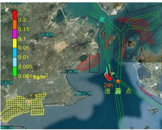
Figure 8.4.37 Impact Scope of Oil Spill Accident Occurred at Point B in Ebb Tide Period in Case of Calm Wind (after 12-21 hours)
