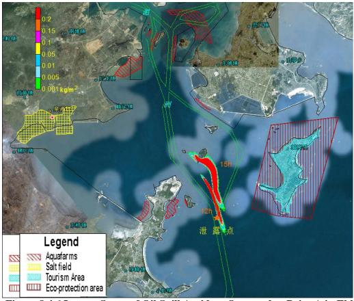
Figure 8.4.6 Impact Scope of Oil Spill Accident Occurred at Point A in Ebb Slack Period in Case of Calm Wind (after 12-15 hours)
