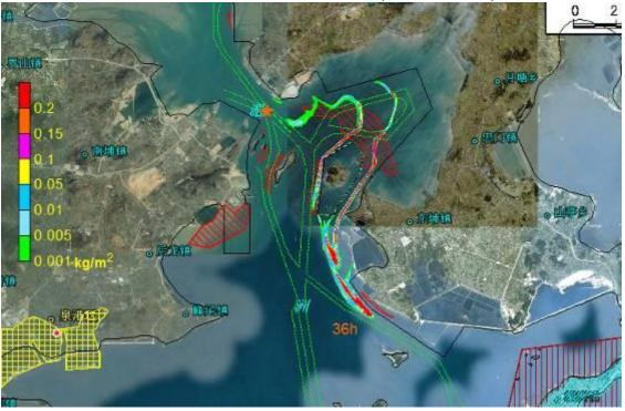
Figure 8.4.96 Impact Scope of Oil Spill Accident Occurred at Point D in Ebb Tide Period in Case of Calm Wind (after 36 hours)
