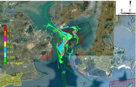
Figure 8.4.90 Impact Scope of Oil Spill Accident Occurred at Point D in Flood Tide Period in Case of Calm Wind (after 36 hours)
