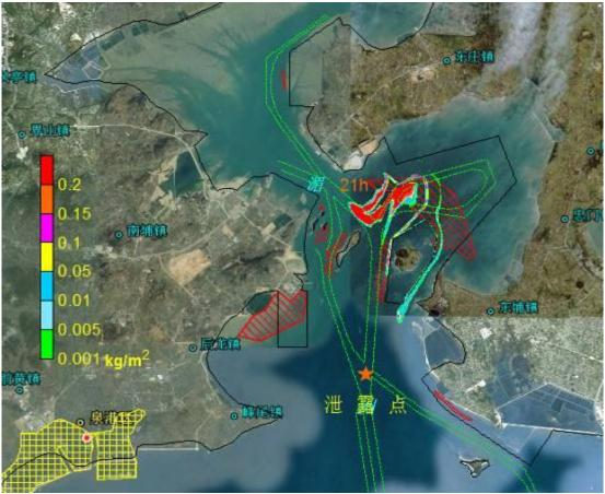
Figure 8.4.28 Impact Scope of Oil Spill Accident Occurred at Point B in Ebb Slack Period in Case of Calm Wind (after 21 hours)
