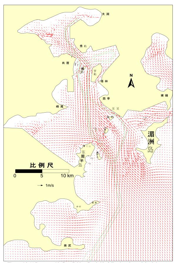
Figure 6.2-11 Down rapids flow field at flood tide following channel dredging
