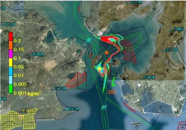
Figure 8.4.62 Impact Scope of Oil Spill Accident Occurred at Point C in Flood
