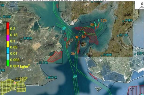
Figure 8.4.74 Impact Scope of Oil Spill Accident Occurred at Point C in Ebb Tide Period in Case of a SSW Wind (after 3-12 hours) 8.4.2.4 Prediction for Leakage Point D
