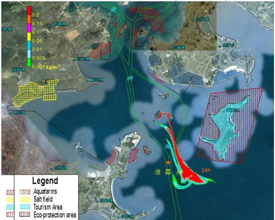
Figure 8.4.9 Impact Scope of Oil Spill Accident Occurred at Point A in Ebb
