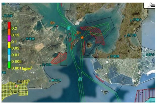
Figure 8.4.69 Impact Scope of Oil Spill Accident Occurred at Point C in Ebb Slack Period in Case of a NE Wind (after 3-6 hours)
