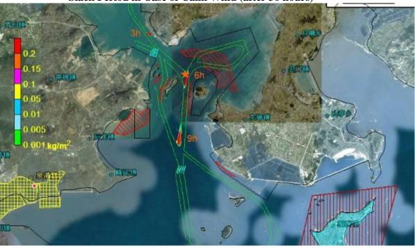
Figure 8.4.57 Impact Scope of Oil Spill Accident Occurred at Point C in Flood Tide Period in Case of Calm Wind (after 3-9 hours)
