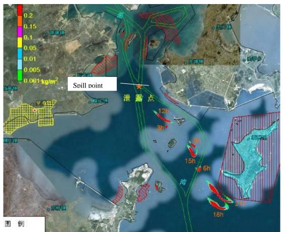
Figure 8.4.22 Impact Scope of Oil Spill Accident Occurred at Point B in Flood Slack Period in Case of Calm Wind (after 3-21 hours)
