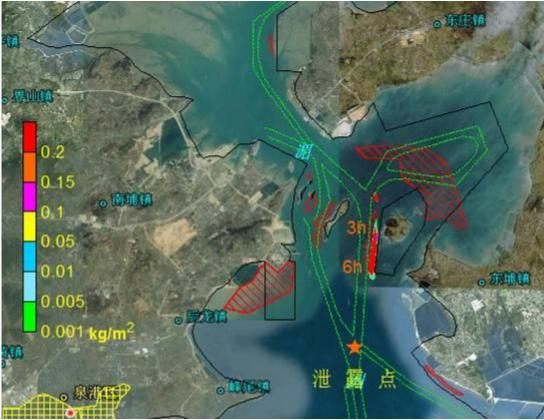
Figure 8.4.46 Impact Scope of Oil Spill Accident Occurred at Point B in Flood Tide Period in Case of a SSW Wind (after 3-6 hours)
