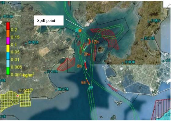
Figure 8.4.75 Impact Scope of Oil Spill Accident Occurred at Point D in Flood Slack Period in Case of Calm Wind (after 3-12 hours)
