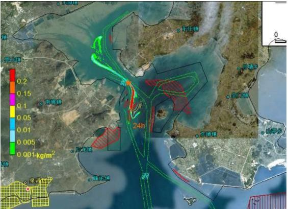
Figure 8.4.77 Impact Scope of Oil Spill Accident Occurred at Point D in Flood Slack Period in Case of Calm Wind (after 24 hours)
