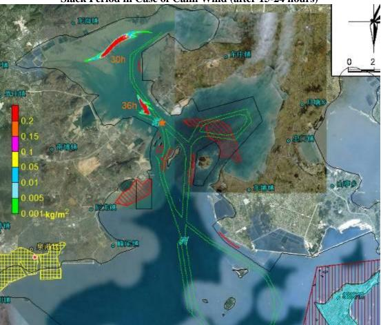
Figure 8.4.82 Impact Scope of Oil Spill Accident Occurred at Point D in Ebb Slack Period in Case of Calm Wind (after 30-36 hours)
