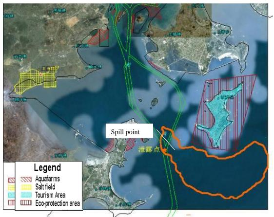
Figure 8.4.106 Maximum Impact Scope of Oil Spill Accident Occurred at Point A in Ebb Tide Period After 36 Hours in Case of Calm Wind
