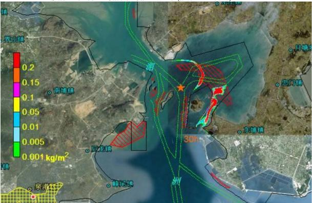
Figure 8.4.55 Impact Scope of Oil Spill Accident Occurred at Point C in Ebb Slack Period in Case of Calm Wind (after 30 hours)
