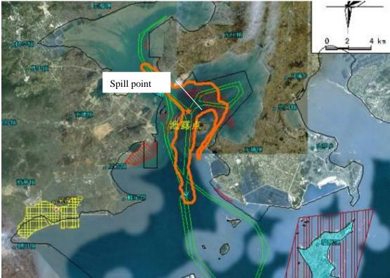
Figure 8.4.114 Maximum Impact Scope of Oil Spill Accident Occurred at Point C in Ebb Tide Period After 36 Hours in Case of Calm Wind
