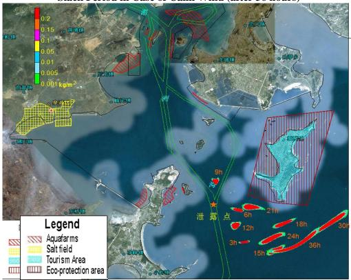
Figure 8.4.12 Impact Scope of Oil Spill Accident Occurred at Point A in Ebb Tide Period in Case of Calm Wind (after 3-36 hours)
