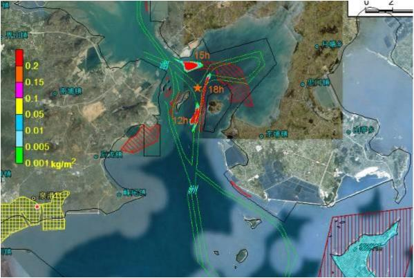
Figure 8.4.58 Impact Scope of Oil Spill Accident Occurred at Point C in Flood Tide Period in Case of Calm Wind (after 12-18 hours)
