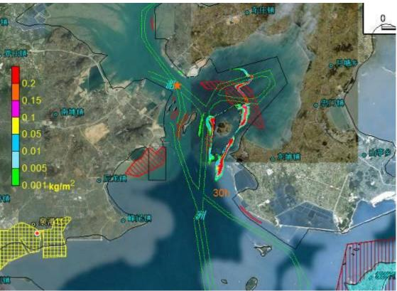
Figure 8.4.95 Impact Scope of Oil Spill Accident Occurred at Point D in Ebb Tide Period in Case of Calm Wind (after 30 hours)
