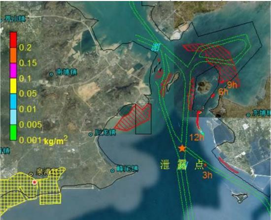
Figure 8.4.47 Impact Scope of Oil Spill Accident Occurred at Point B in Ebb
