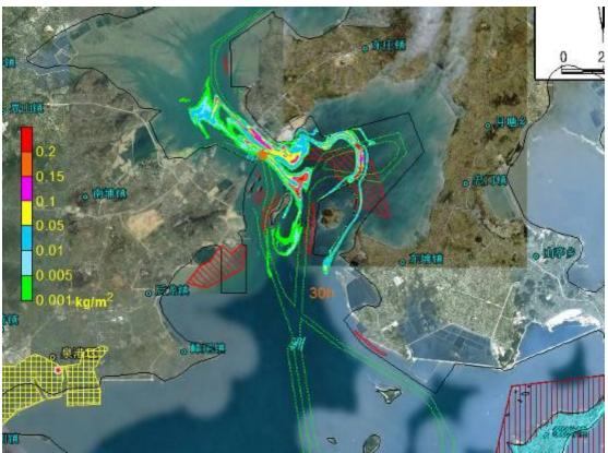
Figure 8.4.89 Impact Scope of Oil Spill Accident Occurred at Point D in Flood Tide Period in Case of Calm Wind (after 30 hours)
