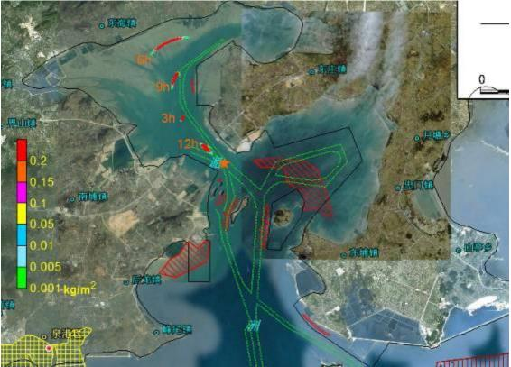
Figure 8.4.80 Impact Scope of Oil Spill Accident Occurred at Point D in Ebb Slack Period in Case of Calm Wind (after 3-12 hours)
