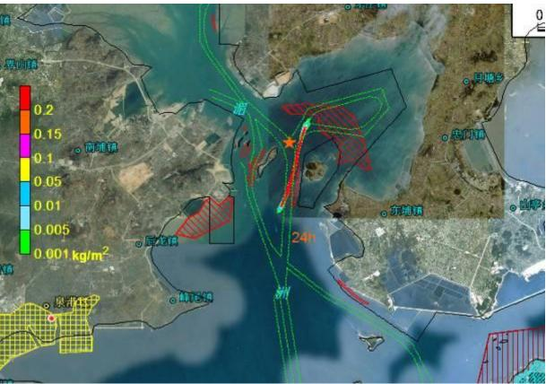
Figure 8.4.65 Impact Scope of Oil Spill Accident Occurred at Point C in Ebb Tide Period in Case of Calm Wind (after 24 hours)
