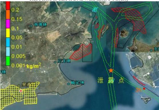
Figure 8.4.44 Impact Scope of Oil Spill Accident Occurred at Point B in Flood Slack Period in Case of a SSW Wind (after 3 hours)
