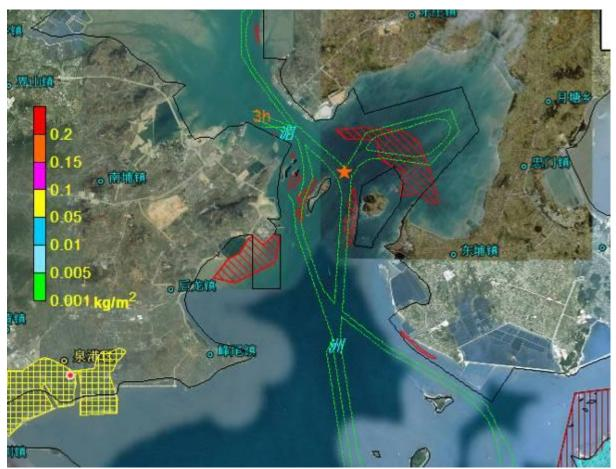
Figure 8.4.71 Impact Scope of Oil Spill Accident Occurred at Point C in Flood
