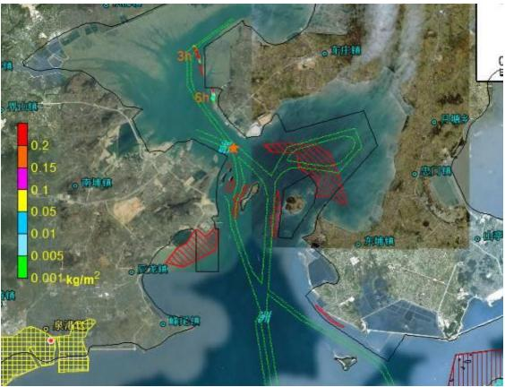
Figure 8.4.101 Impact Scope of Oil Spill Accident Occurred at Point D in Flood Tide Period in Case of a SSW Wind (after 3-6 hours)
