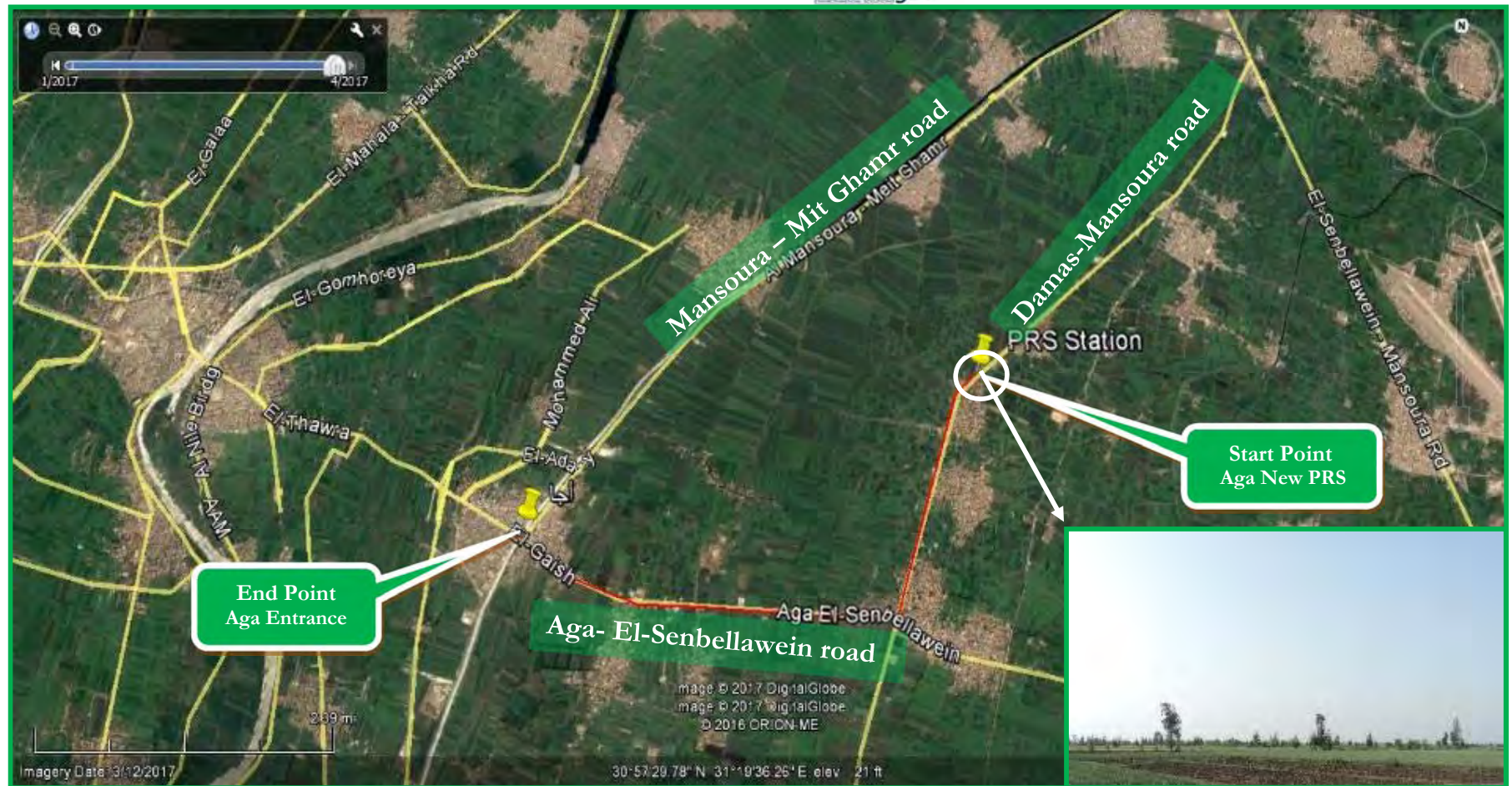
Figure 2-2: The proposed Location of Aga new PRS and pipeline route feeding Aga area
