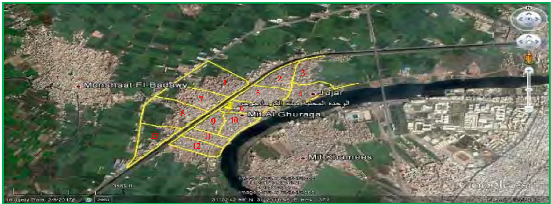
Figure 2-16: Satellite map showing the proposed distribution - network feeding Mit Elkorama, and Gogar Villages
