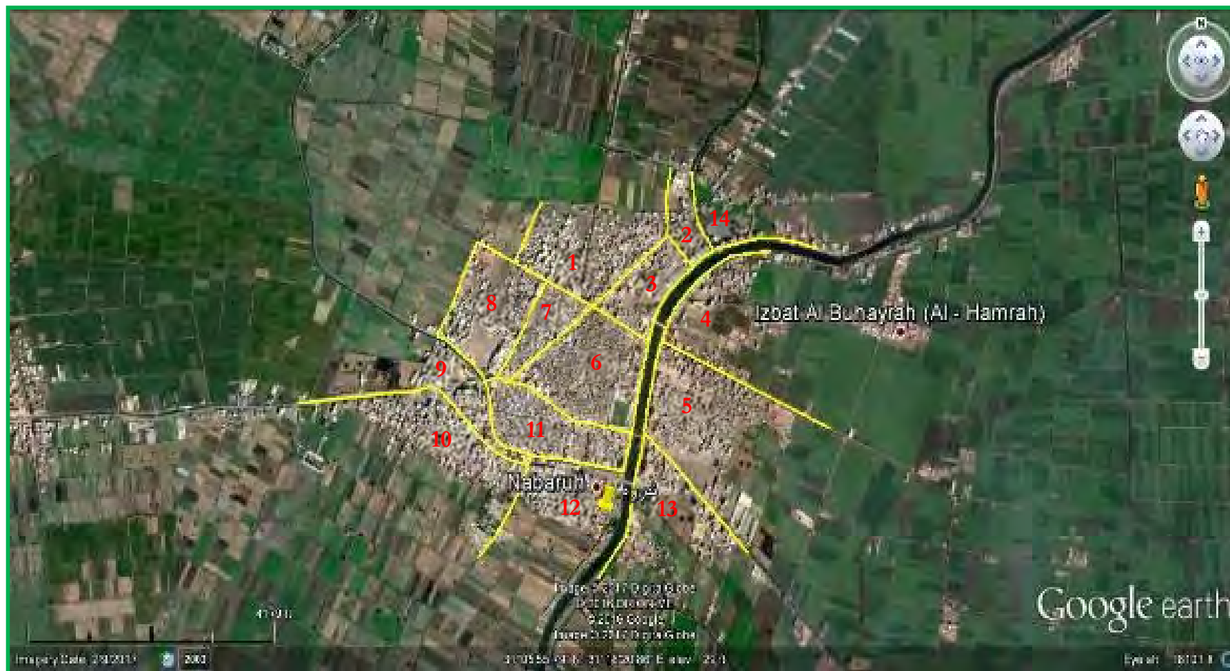
Figure 2-12: Satellite map showing the proposed distribution - network feeding Nabaroh City
