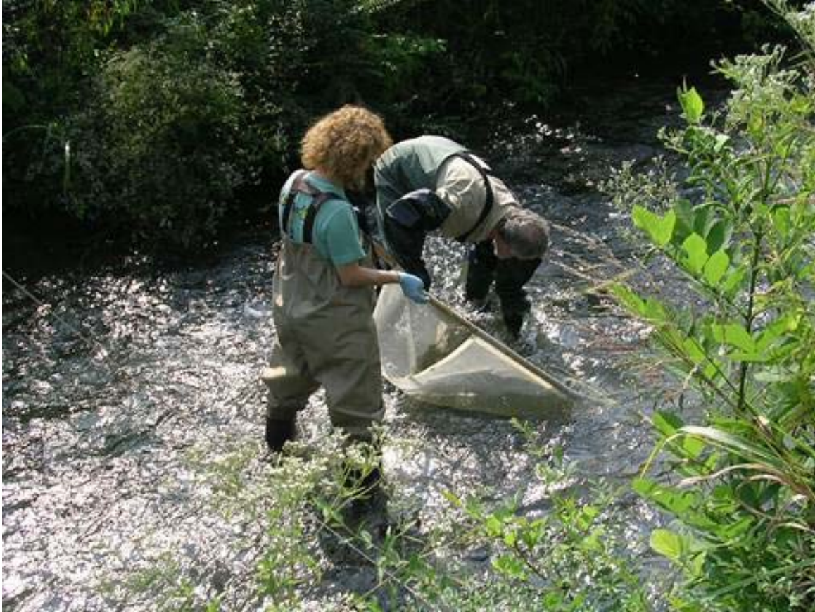
Figure 8.28. Sampling for benthic macroinvertebrates with TDEC protocols.
