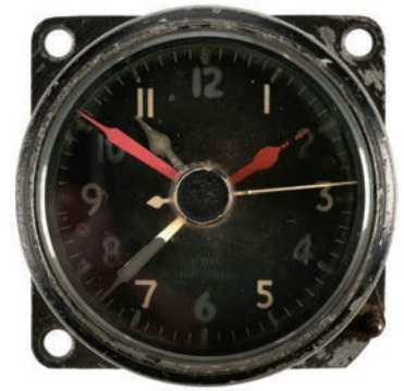
119* WWII. RAF Instrument-Board Time-Clock, circa 1939-45, an Air Ministry 8-day clock, as fitted to Hawker Hurricane & Supermarine Spitfire aircraft inter-alia, stamped AM numbered 22698/44, chapter-ring winder/adjust with strategic time-setting hands and sweep-seconds facility, appears good working order, 2.5 ins (6cm) diameter (1) £200 - £300
