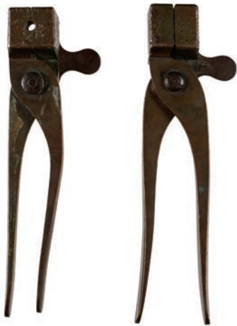
202* Bullet Mould. A Victorian Sporting Rifle Bullet Mould, bronze with steel spruce cutter and spiked ogive 16mm diameter, 22.5cm long, together with another similar bronze with steel spruce cutter and ball mould, 20mm diameter, 23cm long (2) £200 - £300
