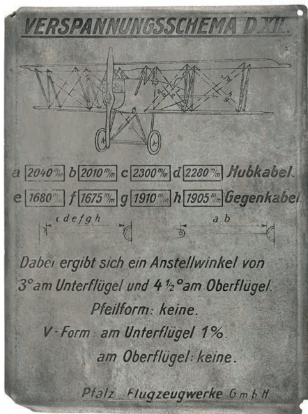
66* Pflaz D.XII. A rare aircraft data plate, circa 1918, the tin aircraft data plate engraved with rigging guide detail, 16 x 12cm A rare piece once fixed to the fuselage of the Pflaz D.XVII circa 1918. The Pflaz D.XII was a German fighter aircraft built by Pflaz Flugzeugwerke. It was designed by Rudolph Gehringer and was supplied in significant numbers toward the end of WWI. It was a highly effective fighter aircraft but hugely overshadowed by the Fokker D.VII. (1) £100 - £150
