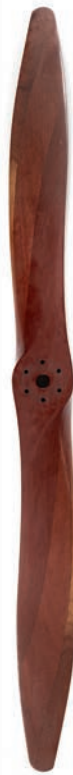
73* Propeller. A small inter-war two-blade aircraft propeller, the laminated mahogany propeller stamped on the boss NP 09 88, the opposite side stamped 25 1 08 64 38, 63cm long (1)
