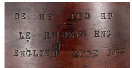
72* Propeller. A WWI DH.5 two-blade propeller, the laminated mahogany propeller stamped on the boss DE H5 110 HP LE RHONE ENG ENGLISH TYPE BOSS, with additional markings numbered 6805, RFC green sheathed tips and boss, a fine example having been in private hands for many years, approximately 260cm long
