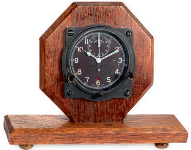
3* Aircraft Clock. A WWII British Mk III aircraft clock by Carley & Clemence Ltd, the 7cm circular black dial with time of trip subsidiary dial, illuminated hands and Arabic numerals, Ref. No. 6A/676A, No. 661-37, Swiss Made movement, mounted on an oak base, 18cm high x 23cm wide (1) £100 - £150
