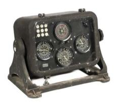
562 **Decometer Unit.** Decca Navigator Mark V Type 134 by the Decca Navigator Co, Ltd, London, circa 1960, black case with glass front enclosing multiple dials and control buttons, on a hinged pivotal support, various data plates including serial number 7560 and serial number 717, 33cm high x approximately 45cm wide (including stand)
