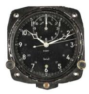
595\* RAF Instrument-board time-clock c1953. A Smiths Air Ministry 8-day "Elapsed-time" chronograph clock as fitted to DH Vampire & Hawker Hunter aircraft inter-alia; Code No. V308, Serial No. 866/53, 6A/3157, Broad-arrow stamped with inscribed plaque to back casing; appears working & in good presentation condition. 3 1/4.in (80mm) dia.
