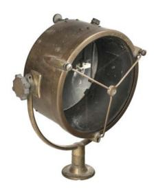
388\* Searchlight. Royal Navy searchlight, probably circa 1950s, the brass case with circular glass protected by 3 bars, on an adjustable pivotal base with handle to the rear for adjusting the direction, 28cm diameter
