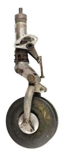
576\* Hawker Typhoon. Rare WWII Hawker Typhoon tail wheel, the 33cm diameter anti-shimmy tyre by Rayon, numbered 5-50-6 TC, the aluminium hub stamped AHO 5007, WH No DG20007, the frame with various stamps including E/G 41, approximately 84cm long overall
