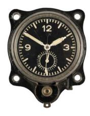
583\* Luftwaffe. WWII German aircraft clock by Junghans, with 50mm circular black dial and luminous arabic numerals, hands and subsidiary seconds dial, black painted case with brass winding crown and four holes for securing to the instrument panel, the screwback enclosing movement stamped J30 BZ serial number 38037, will run if rocked but stops soon after
