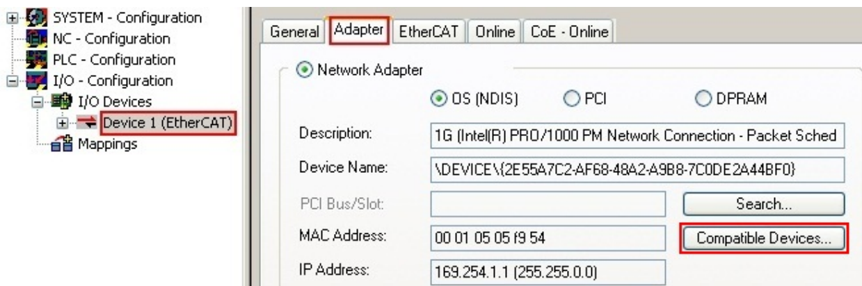
Fig. 116: EtherCAT device properties (TwinCAT 2): click on “Compatible Devices...” of tab “Adapter”
