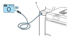
Turn on the camera. Make sure your camera is in PictBridge mode. When the machine has recognized the camera, the LCD shows the following message depending on which mode the machine is in:
