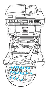
Hold the handles of drum unit when you carry it. DO NOT hold the sides of the drum unit.
