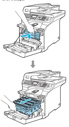
3 Release the gray lock lever (1) that is on the left side of the machine. Lift the front of the drum unit and pull the drum unit completely out of the machine using the green handles on the drum unit.
