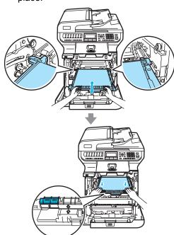
Insert the original orange packing material for locking the belt unit as shown in the illustration.
