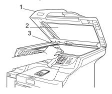
In the ADF unit, clean the white bar (1) and the scanner glass strip (2) underneath it with a soft lint-free cloth moistened with a non-flammable glass cleaner.
