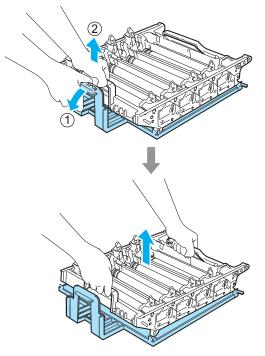
6 Hold the handle of the toner cartridge and slide the toner cartridge into the drum unit. Make sure that you match the toner cartridge color to the same color label on the drum unit, and make sure that you fold down the toner cartridge handle (A) once the toner cartridge is in place. Repeat this for all the toner cartridges.
