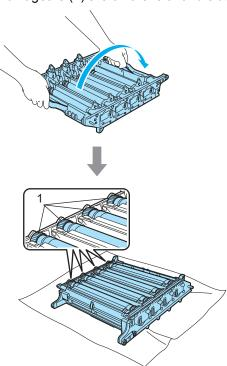
See the print sample to identify the color causing the problem. The color of the spots or toner stain is the color of the drum you should clean. For example, if the spots are cyan, you should clean the drum for cyan. Put the print sample in front of the drum, and the find the exact position of the poor print.
