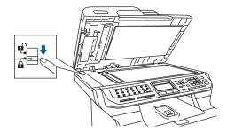
3 Press the front cover release button and then open the front cover.
