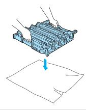
Hold the handle of the toner cartridge and pull it out of the drum unit. Repeat this for all of the toner cartridges.
