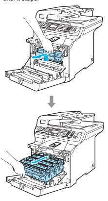
6 Release the gray lock lever (1) that is on the left side of the machine. Lift the front of the drum unit and pull the drum unit completely out of the machine using the green handles on the drum unit.
