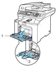
4 Put a blank sheet of A4 or Letter sized paper in the MP tray.
