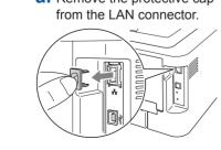
**a.** Remove the protective cap **b.** Connect the network cable to the LAN connector marked with a R symbol and then connect it to a free port on your hub.
