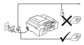
Set the receive mode to External TAD if you have an external answering machine. See Choose a Receive Mode on page 7. Detailed information >> Basic User's Guide: Connecting an external TAD (telephone answering device)
