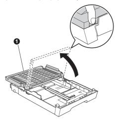
With both hands, gently press and slide the paper length guide **1** and then the paper side guides **2** to fit the paper size.
