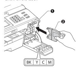
Gently push the back of the ink cartridge marked "PUSH" until it clicks. After all the ink cartridges are installed close the ink cartridge cover.
