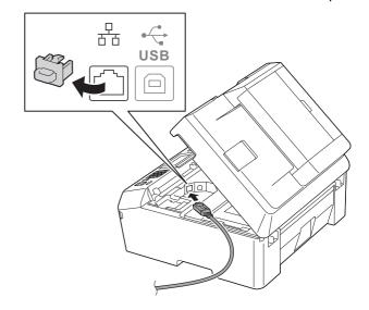
Carefully guide the network cable into the cable channel and out the back of the machine.
