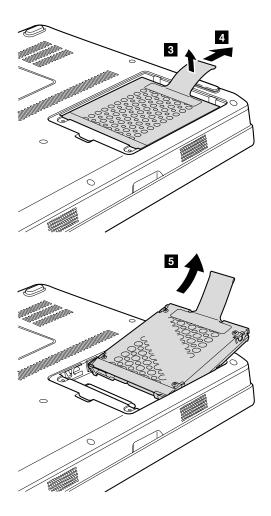
When installing: Make sure that the hard disk drive connector is attached firmly.
