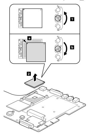
When installing: Place the CPU on the CPU socket **a**, and then rotate the head of the screw in the direction shown by arrow **b** to secure the CPU.
