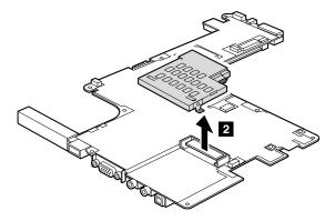
**When installing:** Make sure that the connector is attached firmly, and then fasten the screws.
