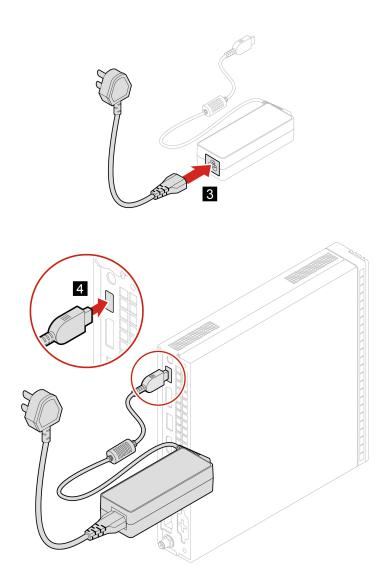
4. Reconnect the external cables and power adapter to the corresponding connectors on the computer.
