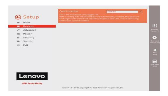
Click on the pulldown menu to enable the Thunderbolt card. The appropriate PCIe slot can be set to Auto, which will allow the BIOS to detect the adapter card on the next boot, or it can be manually set to the desired slot, as shown here:
