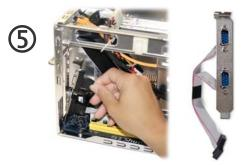
Install the back panel adapter PC7 in a slot of your choice.
