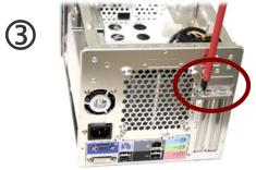
Unfasten the expansion slot bracket screws.
