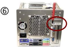
Tighten the bracket screws.
