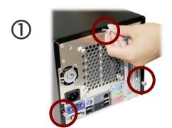
Remove the three thumbscrews of the chassis cover.
