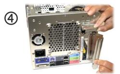
Lift the flap and remove one of the back panel brackets.
