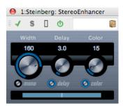
This plug-in will expand the stereo width of (stereo) audio material. It cannot be used with mono files.
