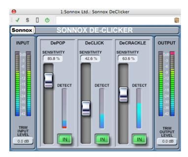
Sonnox DeClicker is one of three plug-ins that form the Sonnox Restoration Toolkit. The tools are not just for restoring old material, but also for removing the clicks, pops, buzzes and background noise that can sometimes accidentally occur in new recordings.
