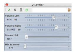
Leveler is useful for correcting an imbalance or adjusting levels between stereo channels, or for mixing down to mono.
