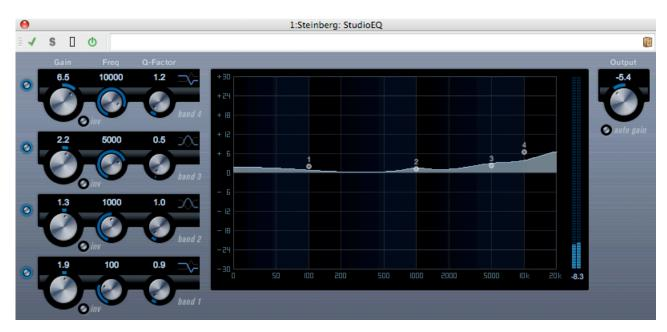
This is a high-quality 4-band parametric stereo equalizer with two fully parametric mid-range bands. The low and high bands can act as either shelving filters (three types), or Parameter Description as a Peak (band-pass) or Cut (low-pass/high-pass) filter.
