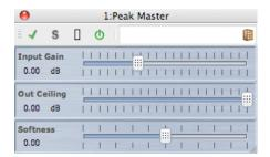
Peak master is a basic plug-in that minimizes peaks in your Audio File, allowing a louder mix without clipping. It is particularly useful in helping to tame very dynamic instruments.
