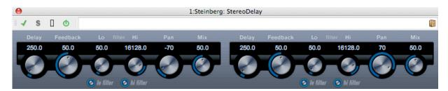
StereoDelay has two independent delay lines with freely specified delay time settings.
