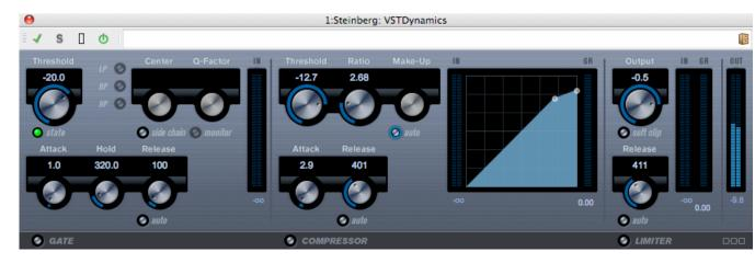
VSTDynamics is an advanced dynamics processor. It combines three separate processors: Gate, Compressor and Limiter, covering a variety of dynamic processing functions. The window is divided into three sections, containing controls and meters for each processor.
