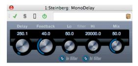
This is a mono delay effect using freely specified delay time settings.
