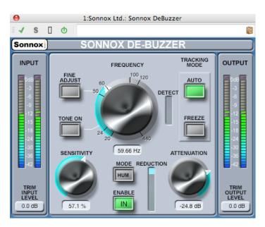
Sonnox DeBuzzer is one of three plug-ins that form the Sonnox Restoration Toolkit. The tools are not just for restoring old material, but also for removing the clicks, pops, buzzes and background noise that can sometimes accidentally occur in new recordings.
