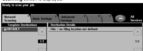
2. Select **Network Scanning** on the touch screen. Ensure that the **Network** Scanning screen is displayed.
