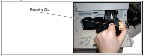
**6.** Hold the empty SMart Kit<sup>TM</sup> Drum Cartridge away from you to avoid spilling any toner residue and dispose of it according to the instructions contained in the new SMart Kit<sup>TM</sup> Drum Cartridge box.
