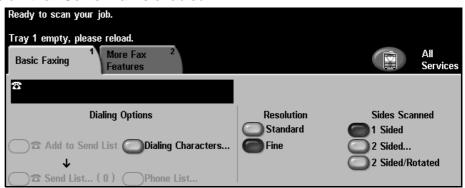
Access to the Basic Faxing features is gained using the **All Services** button on the touch screen. Depending on the options enabled and how your machine has been configured, you may have to select **All Services** and **Fax** to display the Fax feature tabs.
