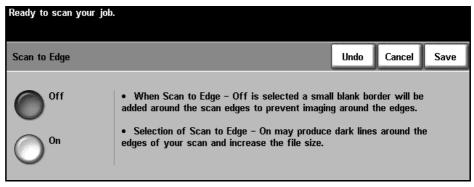
When **Scan to Edge** is switched **Off**, a blank border is automatically added around the edges.
