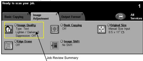
Touch any of the top level buttons to select a feature. To view all the options for a feature, select the option required. Multiple options can be selected for each copy job if required.
