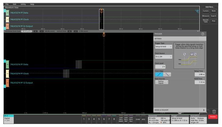
FIGURE 10. Automatic Setup and Hold violation triggering on a 74LVCG74 flip-flop captures many errors.
