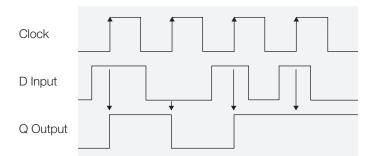
FIGURE 6. Example of flip-flop behavior.
