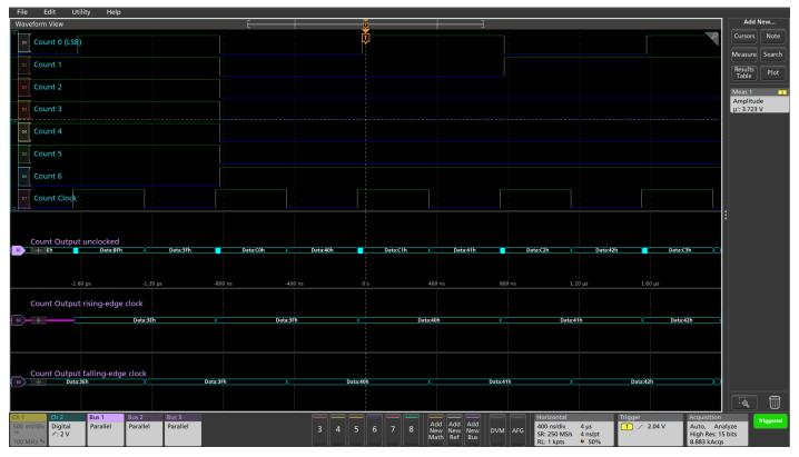
FIGURE 4. Example of a timing acquisition on the MDO/MSO Series. Three parallel buses have been defined and decoded using the device's clock signal.
