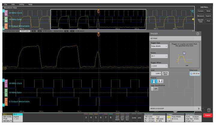
FIGURE 11. Pulse Width triggering captures a narrow glitch on the output of a 74LS74 flip-flop.
