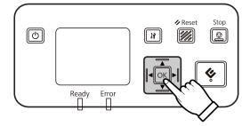
Select **IPv4** with the ▲ up and ▼ down buttons, and then press the **OK** button.
