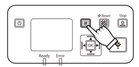
3 Select **Network** with the ▲ up and ▼ down buttons, and then press the **OK** button.
