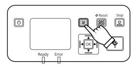
Select **Network** with the ▲ up and ▼ down buttons, and then press the **OK** button.
