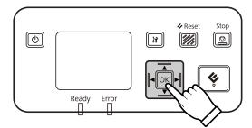
Select **IPv6** - **On** with the ▲ up and ▼ down buttons, and then press the **OK** button.
