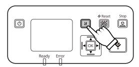
Select **Network** with the ▲ up and ▼ down buttons, and then press the **OK** button.
