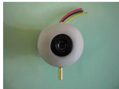
Figure A4. Miniature video cameras are fitted in each eye.
