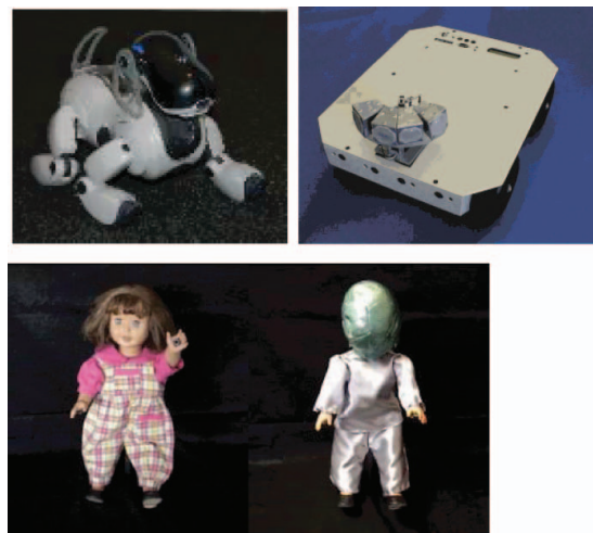
Figure 19. Top row: Non-humanoid, mobile robots used in the Aurora project – Aibo (left, Sony), Labo-1 (right, AAI Canada, Inc.). Bottom row: Different appearances of Robota, the humanoid doll–robot that has been used with children with autism. The 'robot-like' appearance on the right has been shown to be more engaging in first encounters of children with autism compared to Robota, the doll–robot (Robins et al. 2006).
