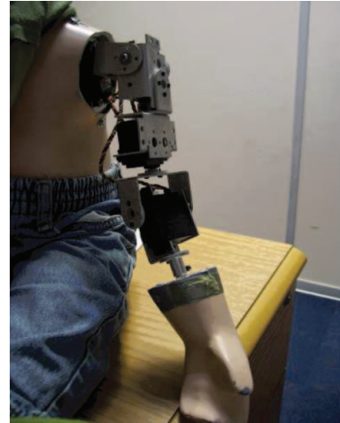
Figure A7. Arm is attached at shoulder end by plates fixed in the dummy body.
