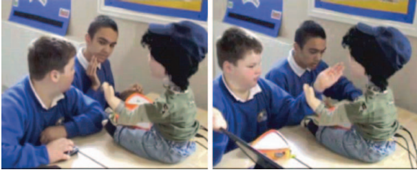
Figure 15. KASPAR mediates child–child interaction in a turn-taking and imitation game: one child controls KASPAR via remote control, the other imitates KASPAR. The children then switch roles.
