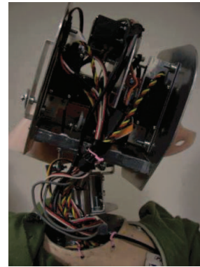
Figure A2. Rear view of head showing wiring and neck joints.
