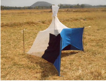
FIGURE 3: Nzi trap. A universal trap able to catch tsetse flies, tabanids, and Stomoxys , especially efficient for large size tabanids.
