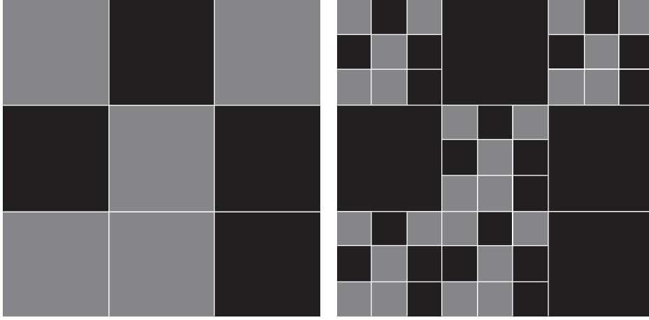
FIGURE 1: Schematic illustration of the solid mass fractal model with E = 2 , n = 3 , and b = 5 . Gray denotes the iterating phase and black denotes the pore phase.
