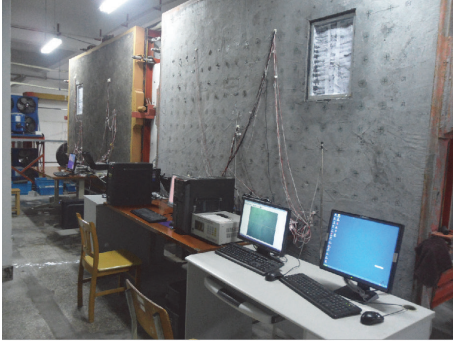
FIGURE 6: Data acquisition system of temperature and strain.
