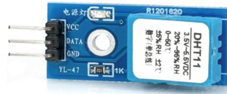
FIGURE 2: Temperature humidity sensor module.
