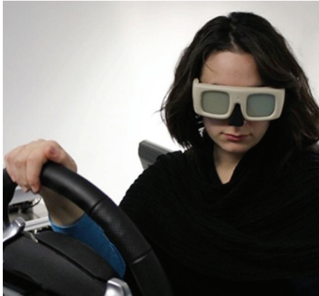
FIGURE 13: Occlusion method with the shutter goggles.
