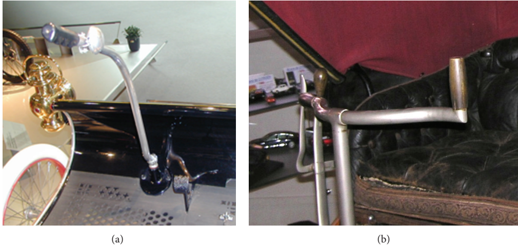
FIGURE 1: Tiller (Oldsmobile 1902 (a)) and bar handle (Peugeot Type 24 1899 (b)) (the author's (MA) photo collection).
