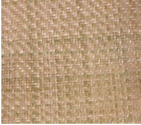
FIGURE 1: Bidirectional roving bamboo fiber.
