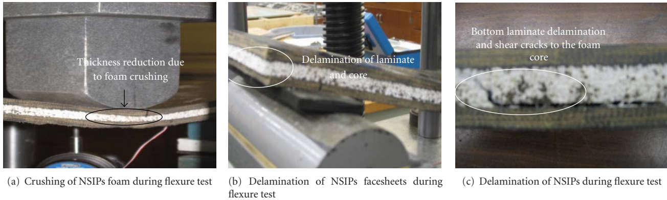
FIGURE 3: Failure modes of NSIPs during flexure test.
