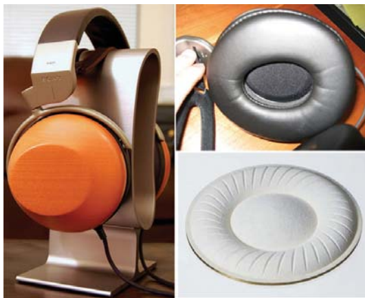
FIGURE 17: Nanocellulose diaphragm used in SONY headphones.
