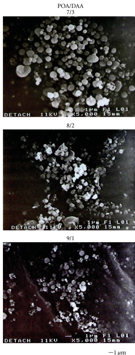
FIGURE 15: SEM images of the nanospheres obtained from the copolymers with POA/DAA of 7/3, 8/2, and 9/1. PA/DAA = 0.5, heterogeneous state.
