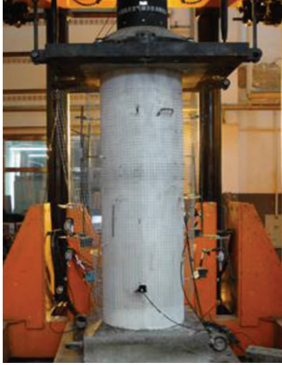
FIGURE 11: Loading and measuring instruments.
