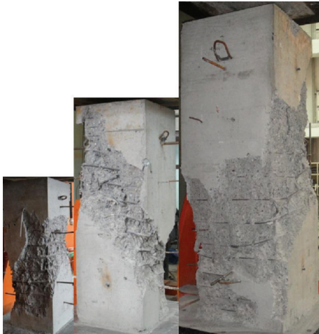
FIGURE 12: Final failure mode of specimens.
