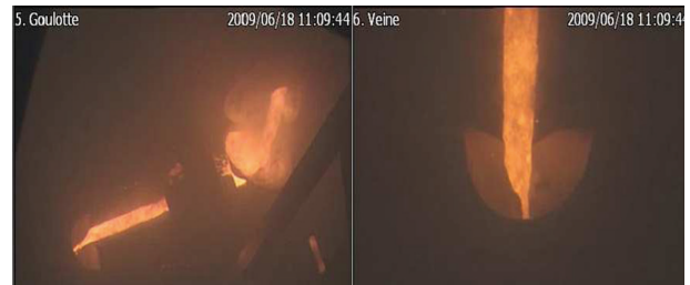
FIGURE 2: Pictures of VULCANO VB-ES-U2 test during corium pouring phase. Left: Corium pouring from the plasma arc rotating furnace (upper right) to the concrete cavity (lower left). Right: Zoom on the concrete hemicylindrical cavity.
